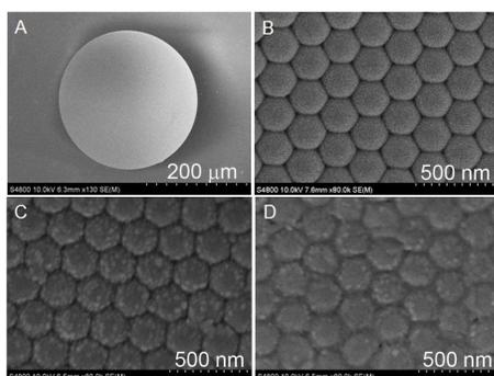
**Fig. 1** SEM image of SPCBs (A), enlarged SEM image of SPCBs (B), Ag-SPCBs (C) and antibody immobilized Ag-SPCBs (D).
