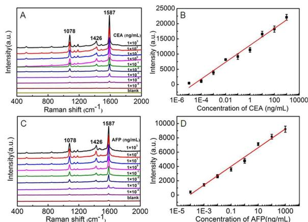
**Fig. 4** SERS spectra of Ag-SPCBs substrates for CEA (A) and AFP (C) with different concentrations of analytes, and calibration curves for CEA (B) and AFP (D) produced at  $1587 \text{ cm}^{-1}$  ( $n = 5$  for each point).
