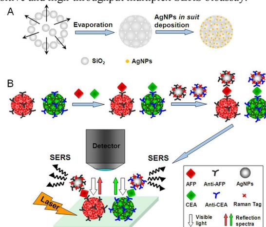
**Scheme 1** The schematic illustration of the fabrication of Ag-SPCBs (A) and multiplex SERS bioassay (B).
