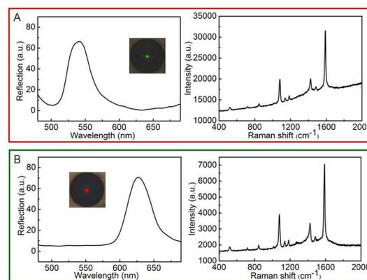
**Fig. 3** The reflection (left) and SERS spectra (right) of CEA sandwich complex immobilized Ag-SPCBs (A) and AFP sandwich complex immobilized Ag-SPCBs (B) at 10 ng/mL concentrations of two tumor markers, insets: the bright filed microscopy images of CEA and AFP sandwich complex immobilized Ag-SPCBs.
