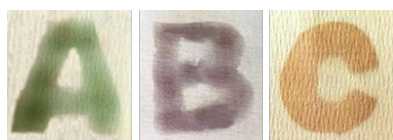
Figure 5. Images of three sheets of white filter paper impregnated with optimal photochromic dye mixture and irradiated by UV-A (A), UV-B (B) (emitted by a 125 W Xe lamp) and UV-C (C) (emitted by a Hg lamp) radiation through negative masks reproducing the letters A, B, and C, respectively.
