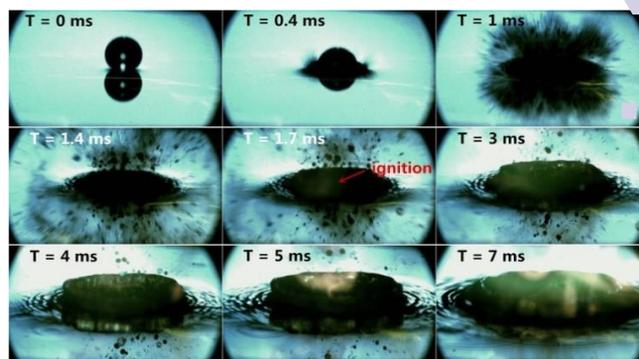
Fig. 2. The droplets tests recorded of HIL **7** with WFNA captured by high speed camera phaton v12 with a long scope microscope; sampling rate is 7000 fps, i.e., the time interval between two frames is 0.143 ms.
