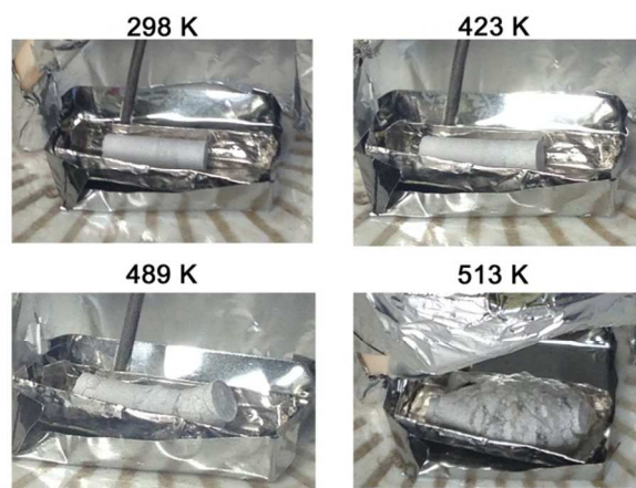
Fig. 2 Images of a mixed pellet of molar composition solvent : \text{KCa}(\text{BH}_4)_3 8.6:1.4 at different temperatures.
