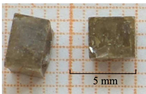
Fig. 1 Photograph of BMT-PT single crystals with rectangular shape.
