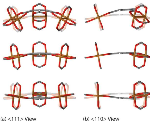
**Fig. 3** Low-energy collective vibration, located at  $81\text{ cm}^{-1}$  (2.4 THz), viewed down the (a)  $\langle 111 \rangle$  and (b)  $\langle 110 \rangle$  directions, showing a 'trampoline-like' motion linked to negative thermal expansion (NTE). Videos of the motions are available in the ESI.
