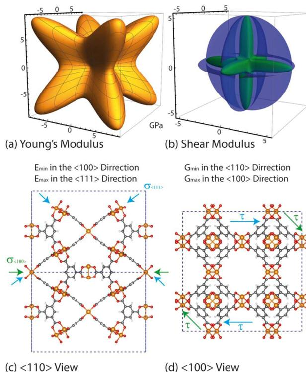
**Fig. 6** (a) Young's modulus representation surface  $E(\vartheta, \varphi)$  in 3-D spherical coordinates, along with (b) shear modulus representation surface  $G(\vartheta, \varphi, \chi)$ . The accompanying structure-property relationships can be seen for (c)  $E_{\min}$  is along the  $\langle 100 \rangle$  axes and  $E_{\max}$  is along the  $\langle 111 \rangle$  axes. (d)  $G_{\min}$  is along the  $\langle 110 \rangle$  axes and  $G_{\max}$  is along the  $\langle 100 \rangle$  axis.
