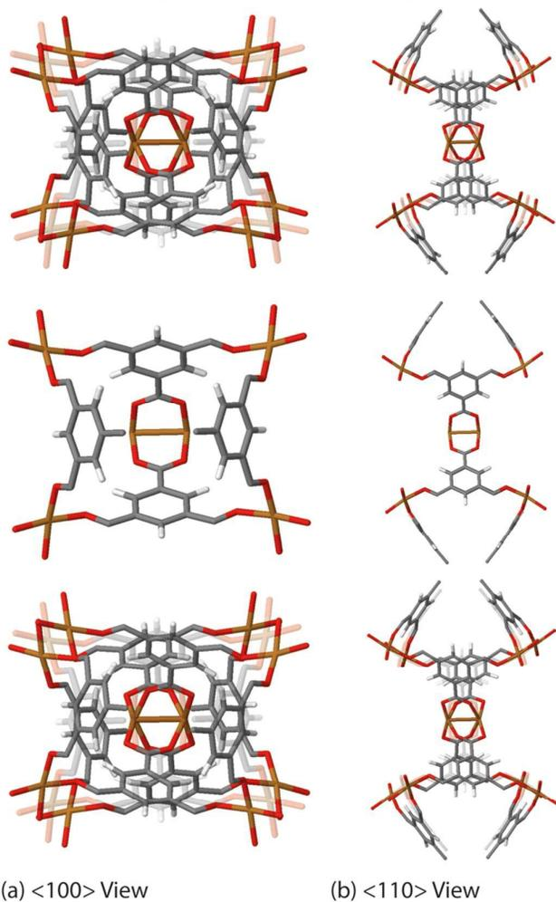
**Fig. 5** Low-energy collective vibration, located at 16  $\text{cm}^{-1}$  (0.5 THz), viewed down the (a)  $\langle 100 \rangle$  and (b)  $\langle 110 \rangle$  directions, showing a cluster rotation mechanism, linked to auxeticity. Videos of the motions are available in the ESI.
