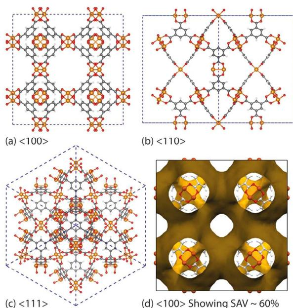
**Fig. 1** Crystal structure of HKUST-1 looking down the (a)  $\langle 100 \rangle$ , (b)  $\langle 110 \rangle$  and (c)  $\langle 111 \rangle$  directions and (d)  $\langle 100 \rangle$  direction displaying the Solvent Accessible Volume (SAV yellow surfaces). Colour code used: copper, orange; carbon grey; oxygen red; hydrogen white.
