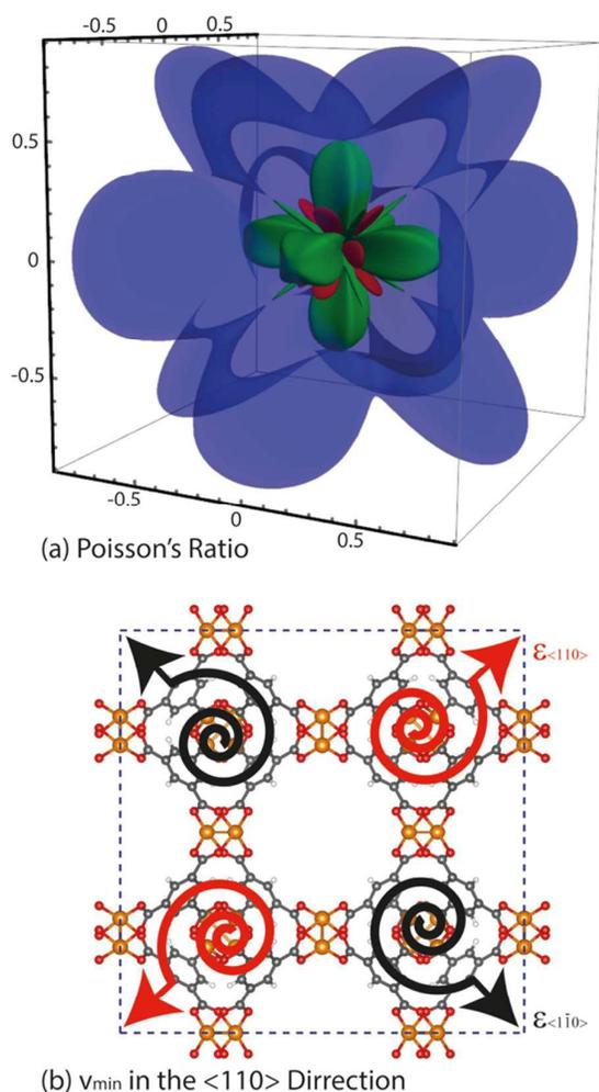
**Fig. 7** Poisson's ratio representation surface  $\nu(\vartheta, \varphi, \chi)$ , where blue signifies the maximum Poisson's ratio and green and red denote the positive and negative minimum Poisson's ratios respectively. (b) Demonstration of the plausible mechanism associated with cluster rotational dynamics responsible for the auxetic response.
