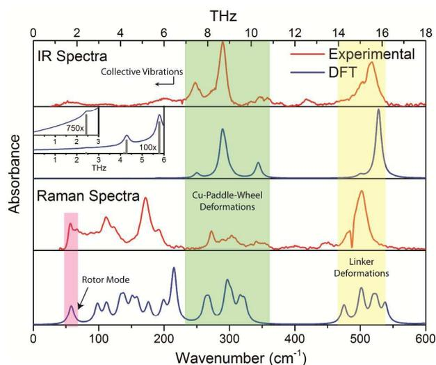
**Fig. 2** Comparison of experimental and theoretical far-infrared (FIR) and Raman spectra in the 0–600 cm<sup>-1</sup> (0–18 THz) region. An empirical 10 cm<sup>-1</sup> FWHM Lorentzian line shape was applied to the DFT spectra to aid in comparison with the experimental data and a bar representation is present for the low intensity IR region below 6 THz.
