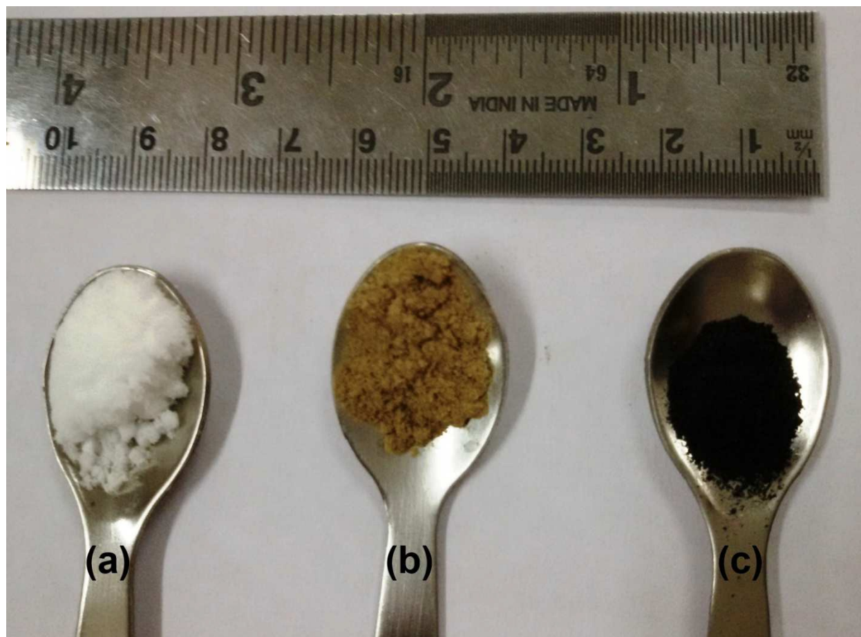
Figure S1. Image depicting the variation in color of powders of (a) “as-fabricated” T-ZnO (white), (b) pretreated T-ZnO after sensitization and activation (yellowish-brown), and (c) Ni-P coated T-ZnO (grayish-black).
