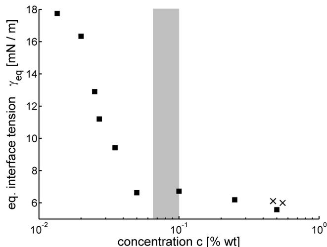
**Fig. 4** Equilibrium interface tensions  $\gamma_{\text{eq}}(c)$ , the shaded region marks the range of critical micelle concentrations from References<sup>33,34</sup>. The two crosses correspond to the measurements published in Ref.<sup>7</sup>.
