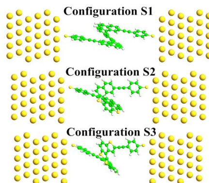
Fig.2 Geometries of the metal-molecule-metal junctions. The spiral-shape molecules are sandwiched between two metallic surfaces of gold. The models of the two-electrode configurations are divided into three regions, including left electrode, scattering region, and right electrode. The sulfur atoms on the both sides of molecules are located at the hollow site on the metallic surfaces.
