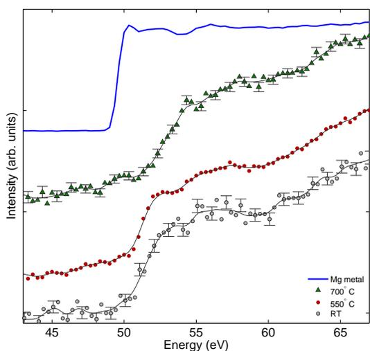
**Fig. 4** Magnesium  $L_{2,3}$  edge spectra in  $Mg_2C_{60}$  after treatments of 30 minutes at different temperature. Reference spectrum for pure magnesium metal is included.
