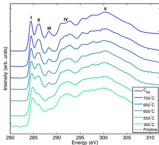
**Fig. 1** X-ray Raman spectra of carbon K edge for pristine and thermally decomposed  $\text{Mg}_2\text{C}_{60}$  samples. Reference spectrum for pure  $\text{C}_{60}$  is included for comparison. The length of the thermal decomposition was 30 minutes.
