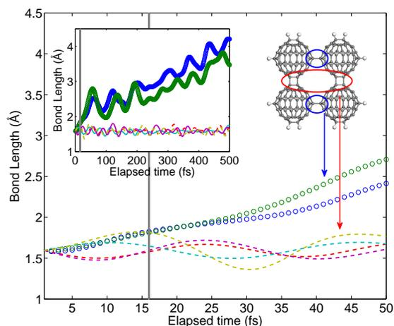
**Fig. 6** Inter-fullerene distance in the molecular dynamics simulation concerning the evolution of a polymer fragment at the temperature of 1000°C: circles correspond to single bonds, lines to the network of double bonds. Vertical thin lines mark the range of stabilization during the simulation. Inset shows results of the whole simulation up to 0.5 ps. The simulation unit and the bonds concerned are shown.
