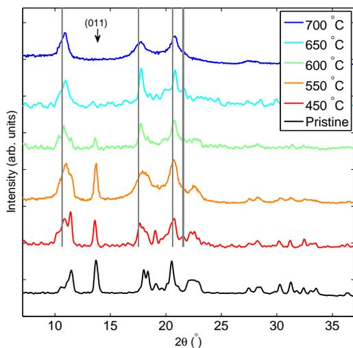
**Fig. 2** X-ray diffraction after thermal treatments of  $\text{Mg}_2\text{C}_{60}$ . The length of the applied thermal treatments was 30 minutes. Vertical thin grey lines correspond to the reflection of pure  $\text{C}_{60}$ .
