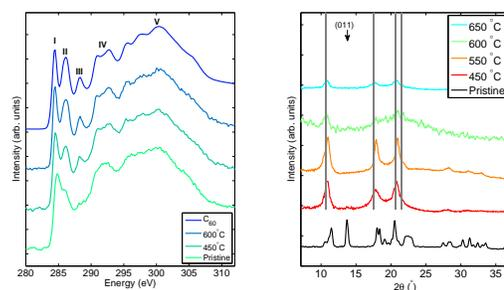
**Fig. 3** Carbon K edge XRS (left panel) and X-ray diffraction (right panel) measurements after extended thermal treatments of  $\text{Mg}_2\text{C}_{60}$ . The length of the applied thermal treatments was 60 minutes.
