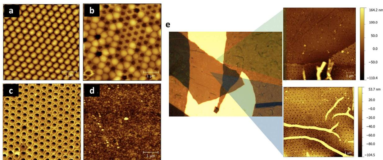
**Figure 23. Creation of free-standing Janus mesoporous virus film.** Topographical tapping mode AFM images illustrate the initial formation of close-packed PS microspheres (a), partial removal of PS spheres (b) after patterned poly(pyrrole-co-pyrrole-3-carboxylic acid) electropolymerization (c), and a non-patterned film (d). e) Optical microscope image (480 μm by
