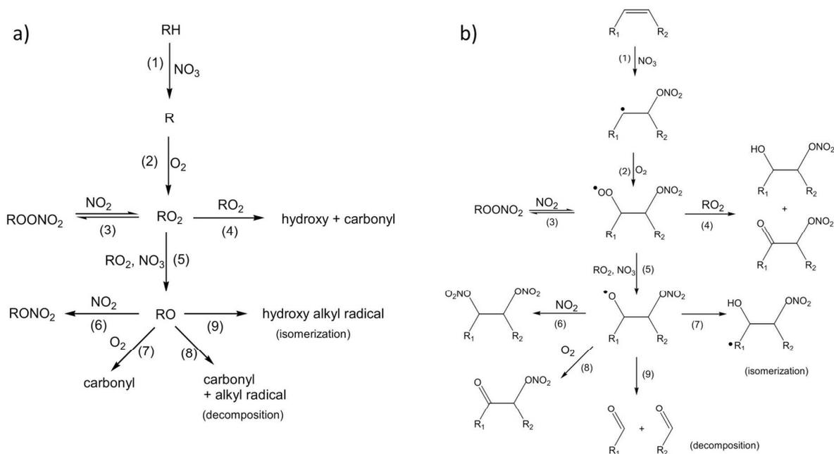
**Figure 8.** Proposed mechanism for addition of  $\text{NO}_3$  to an (a) alkane and (b) alkene surface in the presence of  $\text{NO}_2$  and  $\text{O}_2$ . Copyright 2009 Wiley. Used with permission from Gross, S.; Bertram, A. K., Products and kinetics of the reactions of an alkane monolayer and a terminal alkene monolayer with  $\text{NO}_3$  radicals. *Journal of Geophysical Research: Atmospheres* **2009**, *114*, D02307.
