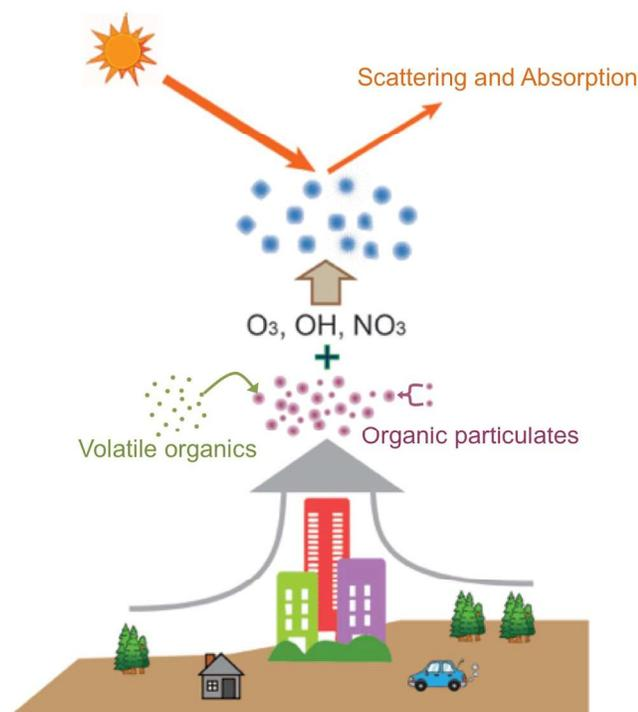
**Figure 1.** Schematic illustration of the generation and transformation of organic particles in the atmosphere. Particles can form and grow from biogenic and anthropogenic emission products, adsorption of volatile organics onto surfaces, coagulation of carbonaceous nanoparticles, and reactions of atmospheric oxidants on the surfaces of existing organic particles. These particles can affect the balance of incoming and outgoing solar radiation.
