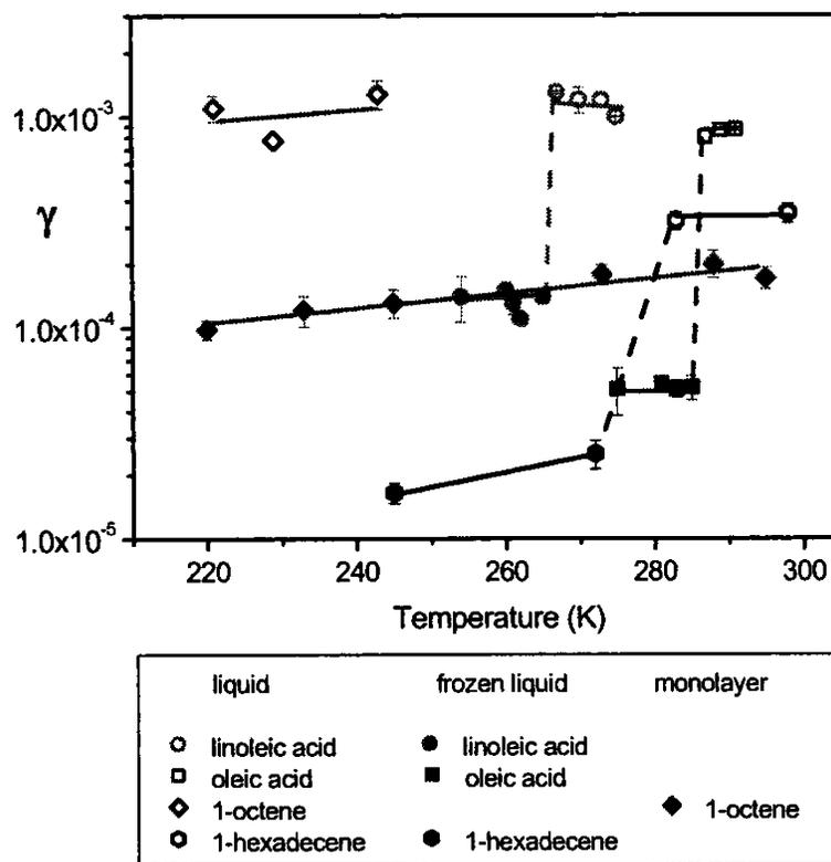
**Figure 4.** Ozone reactive uptake coefficients,  $\gamma$ , vs. temperature (K) for several organic liquids, frozen liquids, and a monolayer.<sup>82,83</sup> The dashed lines show an order of magnitude difference in uptake coefficient between liquid and frozen samples. Reprinted (adapted) with permission from *J. Phys. Chem. A*, 2002, 106, 6469-6476. Copyright 2002 American Chemical Society.
