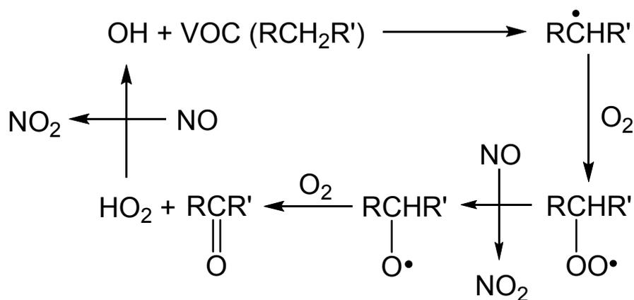
**Scheme 2.** Generation of NO<sub>2</sub> during typical oxidation of volatile organic compounds (VOC) by OH.
