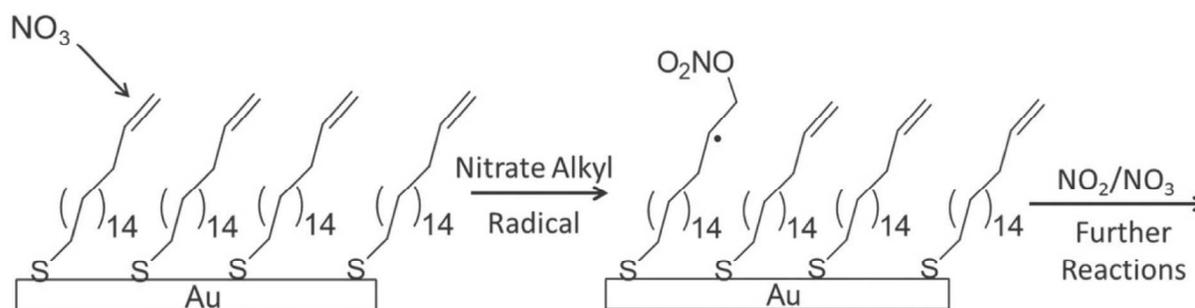
**Figure 9.** A scheme for the reaction of nitrate radical with a vinyl-terminated self-assembled monolayer. Positioning of the  $\text{C}=\text{C}$  bond at the gas-surface interface affords a higher reaction probability than in experiments with a submerged  $\text{C}=\text{C}$  bond (as shown in Figure 5 for  $\text{O}_3$  reactions). Reproduced from Ref. 115 with permission from the PCCP Owner Societies.
