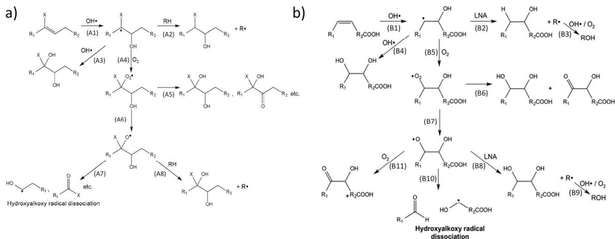
**Figure 11.** Proposed mechanism for addition of OH to (a) squalene, a branched alkane, and (b) linolenic acid, a linear, unsaturated carboxylic acid, in the presence of O<sub>2</sub>. Copyright 2009 Wiley. Reprinted (adapted) with permission from a) *J. Phys. Chem. A*, 2014, 118, 4106. b) *J. Phys. Chem. A*, 2014, 118, 11555. Copyright 2014 American Chemical Society.
