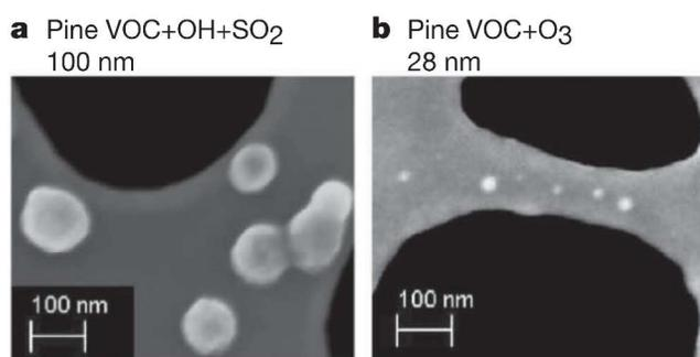
**Figure 2.** SEM images of SOA particles of different sizes resulting from the oxidation of pine-seedling volatile organic compound (VOC) emissions following a) OH-initiated oxidation in the presence of SO<sub>2</sub>, and b) O<sub>3</sub>-initiated oxidation. The white spots are SOAs supported on a lacey carbon grid (black regions). Reprinted with permission from Macmillan Publishers Ltd.: *Nature* **2010**, 467, 824. Copyright 2010.
