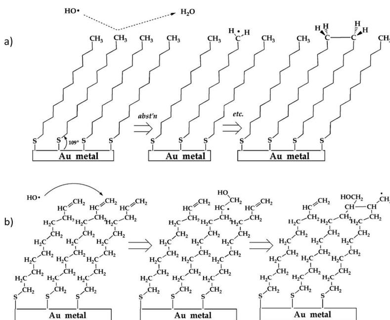
**Figure 12.** Mechanisms of OH + a) alkane and b) alkene-terminated SAM surfaces proposed by D'Andrea et al. In a), isolated alkyl radicals cannot diffuse due to SAM stability. Subsequent OH collisions can result in further radical generation and cross-linking dimerization. In b), polymerization results in a cross-linked alcohol. Reprinted (adapted) with permission from *J. Phys. Chem. B*, 2008, 112, 535. Copyright 2008 American Chemical Society.
