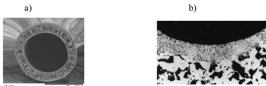
Fig. 3 The hierarchical structure is produced by double mantle spinning. a) Double mantle spun poly lactide hollow fiber membranes for the use in hemodialysis [4]. b) Sintered metal membrane that combines high permeability and very low pressure drop, yet retaining all the advantages of sintered metal filters [5].
