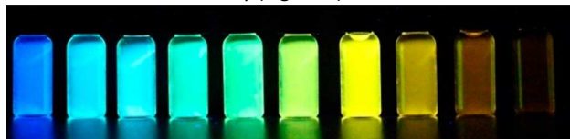
Figure 3. Emission solvatochromism of compound 26b (recorded in cyclohexane, toluene, THF, EtOAc, acetone, \text{CH}_2\text{Cl}_2 , MeCN, iPrOH, EtOH, MeOH (from left to right); T = 293 K; c(\mathbf{26b}) = 10^{-4} M; \lambda_{\text{excit}} = 356 nm, hand-held UV lamp). Reprinted with permission from J. Org. Chem. , 2014 , 79 , 3296–3310. Copyright 2014 American Chemical Society.
