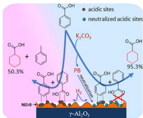
Fig. 9 Proposed mechanism for the hydrogenation of BA with or without K_2CO_3 .
