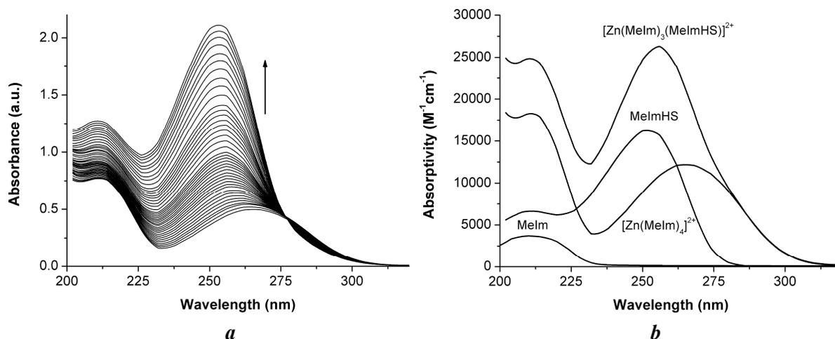
**Fig. 7** (a) Selected spectra collected during the titration of  $[\text{Zn}(\text{MeIm})_4]^{2+}$  ( $8.53 \times 10^{-5} \text{ M}$ ) with MeImHS ( $3.50 \times 10^{-4} \text{ M}$ ) from 0 to 4 MeImHS/ $[\text{Zn}(\text{MeIm})_4]^{2+}$  molar ratio; (b) pure spectra of MeIm, MeImHS,  $[\text{Zn}(\text{MeIm})_4]^{2+}$ , and  $[\text{Zn}(\text{MeIm})_3(\text{MeImHS})]^{2+}$ ; [ $T = 25 \text{ }^\circ\text{C}$ , 0.1 M buffer solution pH 9 (borax / hydrochloric acid), 1 cm optical path length].
