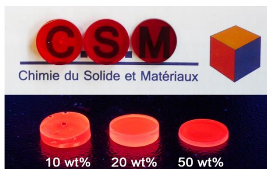
Figure 2. Digital photographs of the pellets PMMo10, PMMo20 and PMMo50 under visible (above) and under UV ( \lambda_{\text{exc}} = 365 \text{ nm} )
