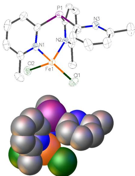
**Figure 6:** Structure of  $[P(2-py)_3]FeCl_2$ ·toluene (**5**-toluene) (top) and the space filling diagram (bottom). Lattice-bound toluene molecules and hydrogen atoms are omitted for clarity. Displacement ellipsoids are drawn at the 50 % probability level.
