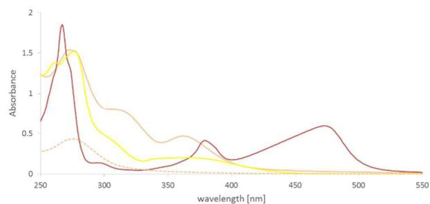
Figure 4: UV-visible spectra of **4** (red, in  $\text{CH}_2\text{Cl}_2$ ), **5**-toluene (orange, in  $\text{CH}_2\text{Cl}_2$ ), **6**-2THF (dotted orange, in MeOH) and **7** (yellow, in  $\text{CH}_3\text{CN}$ ). All spectra were recorded at a concentration of  $5.0 \cdot 10^{-5} \text{ mol L}^{-1}$ . Background solvent corrections were applied.
