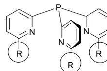
**Figure 2:** The P(2-py')<sub>3</sub> ligand set and the steric effects of substitution of the pyridyl rings at the 6-position.
