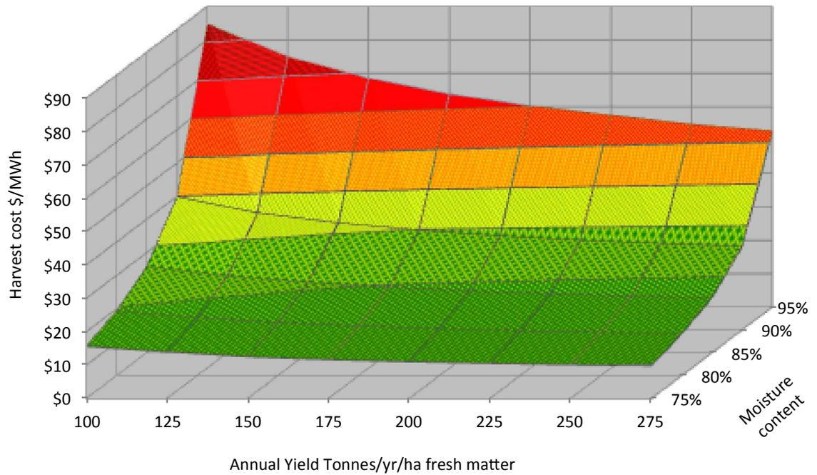
**Figure 1** Modelled costs of harvesting and hauling a CAM crop for a 2.4 MW(e) AD plant based on actual costs of harvesting and hauling.
