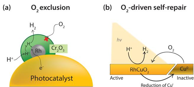
**Figure 10.** (a) Schematic representation of O<sub>2</sub> exclusion by a Cr<sub>2</sub>O<sub>3</sub> layer loaded on a Rh cocatalyst for photocatalytic water splitting.<sup>110</sup> (b) Illustration of O<sub>2</sub>-driven self-repair after photocorrosion of a CuRhO<sub>2</sub> electrode to form inactive Cu<sup>0</sup>.<sup>111</sup>
