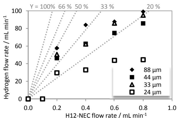
**Fig. 4** – Dehydrogenation of H12-NEC – effect of H12-NEC flow variation on hydrogen yields: Reaction temperature: 260 °C; catalyst: 24 μm, 33 μm, 44 μm, 88 μm; 30 catalyst spheres; platinum mass between 0.36-1.87 mg.
