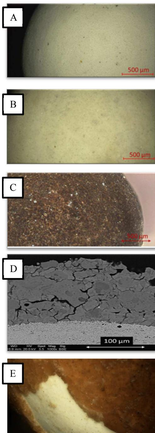
**Fig. 2** - Sphere coating: Top down: (A) – Uncoated; (B) – Coated; (C) – Impregnated; (D) – Coating layer; (E) - Impregnated coating, partially removed.
