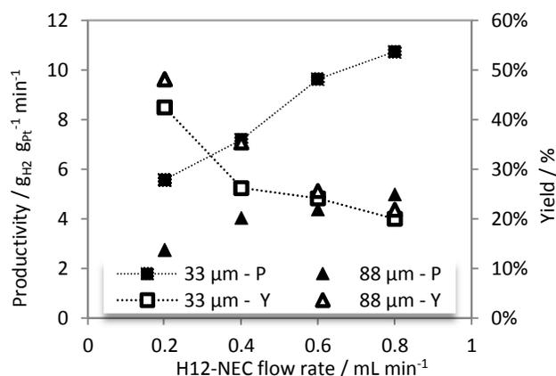
**Fig. 6** – Productivity and corresponding yield: Reaction temperature:  $260 \text{ }^\circ\text{C} \pm 1 \text{ }^\circ\text{C}$ ; catalysts:  $33 \mu\text{m}$ ,  $88 \mu\text{m}$ ; 30 catalyst spheres; Pt mass: 0.82 mg and 1.87 mg.
