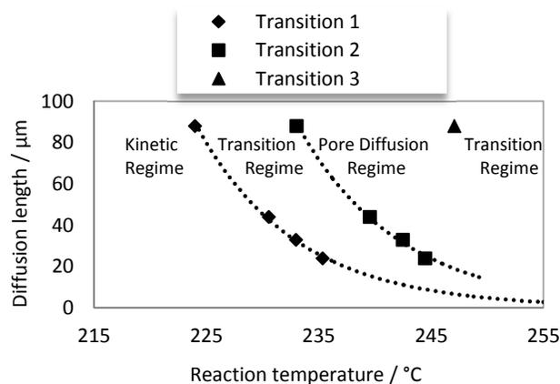
35 **Fig. 11** – Reaction regime map: Reaction temperature: 224  $^{\circ}\text{C}$  – 261  $^{\circ}\text{C}$ ; H12-NEC flow rate 0.6  $\text{mL min}^{-1}$ ; Catalysts: 24  $\mu\text{m}$ , 33  $\mu\text{m}$ , 44  $\mu\text{m}$ , 88  $\mu\text{m}$ ; 30 catalyst spheres; Platinum mass: 0.36–1.87 mg.
