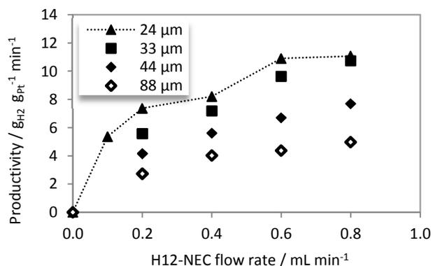
**Fig. 5** - Catalyst productivity as function of H12-NEC flow rate: Reaction temperature: 260 °C ± 1 °C; catalysts: 24 μm, 33 μm, 44 μm, 88 μm; 30 catalyst spheres; Pt mass in reactor: 0.36-1.87 mg; productivity defined as gram H<sub>2</sub> released per gram Pt.
