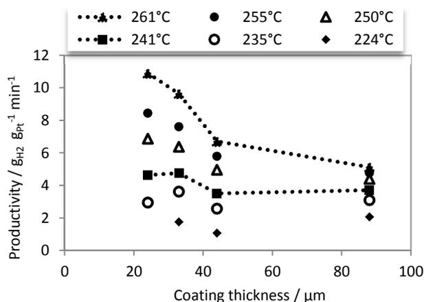
**Fig. 7** – Productivity as a function of diffusion length: Reaction temperature:  $224 \text{ }^\circ\text{C} - 261 \text{ }^\circ\text{C}$ ; H12-NEC flow rate  $0.6 \text{ mL min}^{-1}$ ; catalysts:  $24 \mu\text{m}$ ,  $33 \mu\text{m}$ ,  $44 \mu\text{m}$ ,  $88 \mu\text{m}$ ; 30 catalyst spheres; Pt mass: 0.36-1.87 mg.
