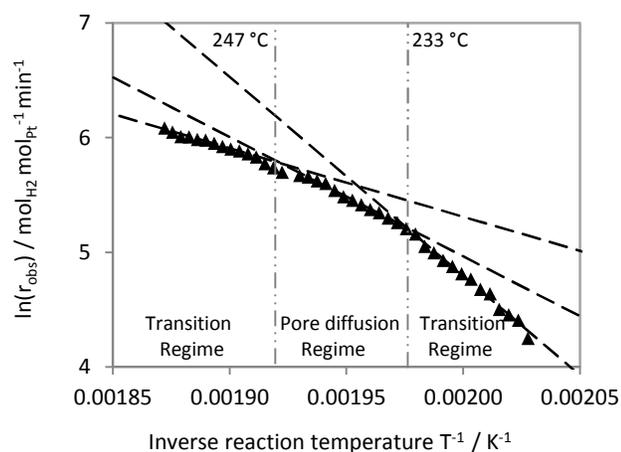
5 **Fig. 10** - Arrhenius plot for the 88  $\mu\text{m}$  catalyst: Reaction temperature: 224  $^{\circ}\text{C}$  – 261  $^{\circ}\text{C}$ ; H12-NEC flow rate 0.6  $\text{mL min}^{-1}$ ; active layer of catalyst: 88  $\mu\text{m}$ ; 30 catalyst spheres; Pt mass= 1.87 mg;  $\text{H}_2$ -yield < 33 %; constant slopes (pore diffusion regime vs. transition regimes) are displayed as dashed lines.
