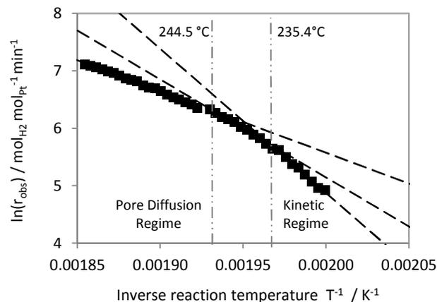
**Fig. 9** – Arrhenius plot for the 24 μm catalyst: Reaction temperature: 224 °C – 261 °C; H12-NEC flow rate 0.6 mL min<sup>-1</sup>; active layer of catalyst: 24 μm; 30 catalyst spheres; Pt mass 0.36 mg; H<sub>2</sub>-yield < 33 %; constant slopes (kinetic vs. pore diffusion regime) are displayed as dashed lines.
