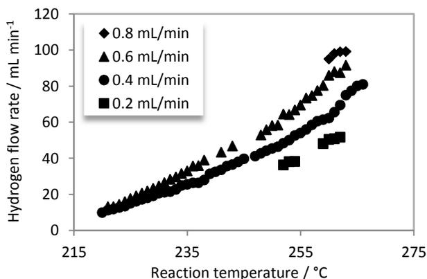
**Fig. 3** - Dehydrogenation of H12-NEC as a function of temperature: Reaction temperature between 220 °C and 266 °C; H12-NEC flow rates between 0.2 mL min<sup>-1</sup> and 0.8 mL min<sup>-1</sup>; catalyst spheres with 33 μm coating thickness; 30 spheres applied
