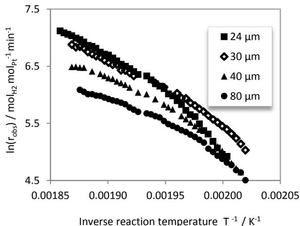
**Fig. 8** – Arrhenius plot derived from all experimental data obtained in this study: Reaction temperatures: 224 °C - 261 °C; H12-NEC flow rate 0.6 mL min<sup>-1</sup>.
