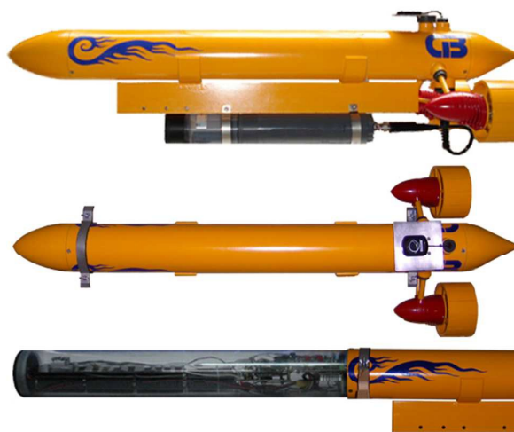
Fig. 2 The USV is equipped with a water quality sonde and electronic components; the latter were housed in a sealed acrylic container.
