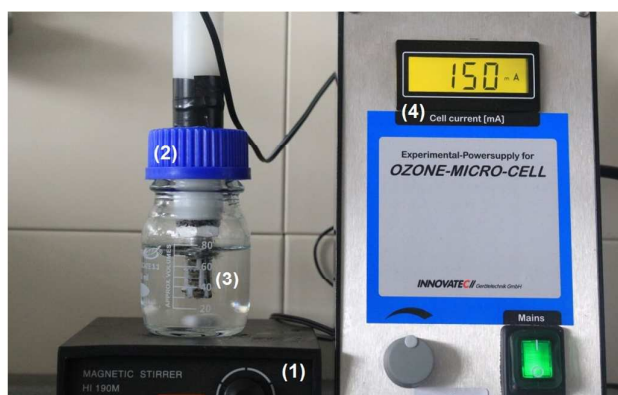
Figure 2 Electrochemical apparatus. Magnetic stirrer (1); 100-mL-flask (2), the lid is prepared with a hole fitting the bar to which the microcell (3) is attached. In this figure the microcell is assembled with four cell hearts. The supply current is adjusted at the control unit (4).
