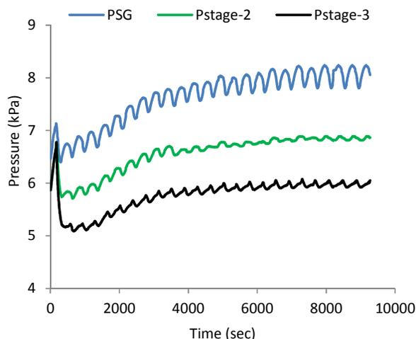
Figure 5: Measured pressure profiles of the key components of MEAD cycle.
