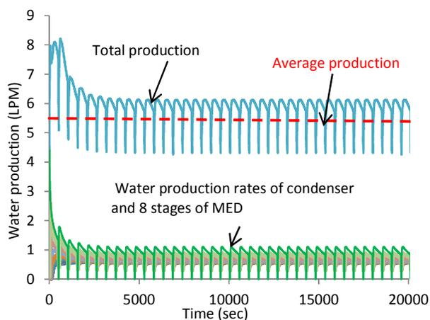
Figure 8: Water production profiles of MEAD by exploiting the total recovered latent energy of condenser.
