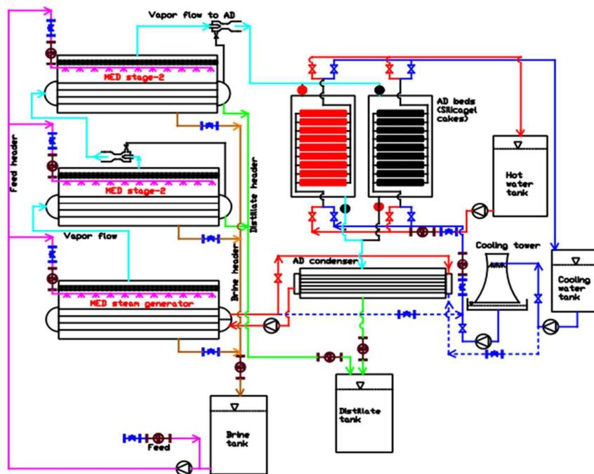
Figure 3(a): Detailed flow schematic of a 3-stages ME-AD cycle with AD heat recovery loop
