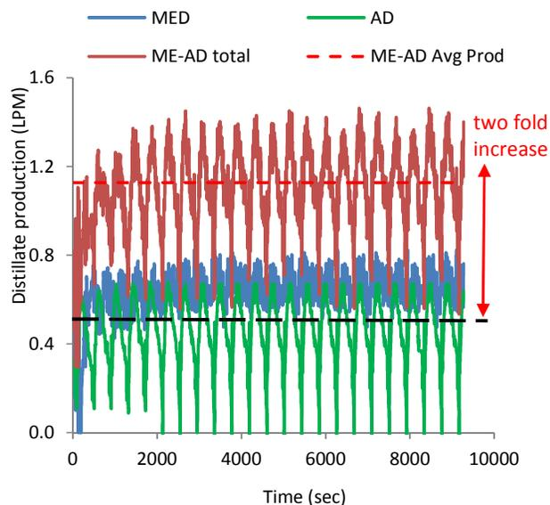
Figure 6: The combined and individual distillate production of the MEAD cycle.
