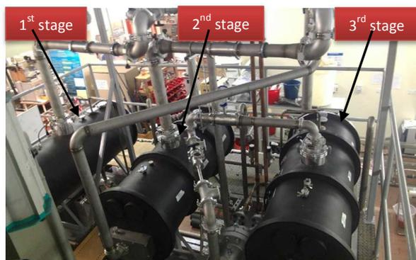
Figure 3(b): A 3-stage ME-AD experimental facility at NUS's adsorption desalination laboratory.
