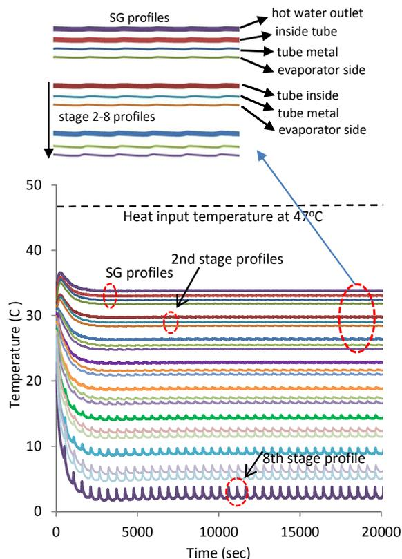
Figure 7: A projected 8-stages MEAD temperature profiles for a full exploitation of the recovered energy of condenser.
