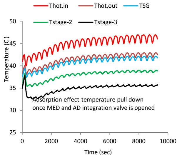
Figure 4: Measured temperature profiles of key components of a MEAD cycle.
