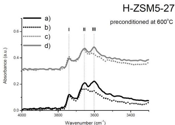
**Fig. 5** DRIFT spectra of H-ZSM5-27 catalyst at 280°C: a) fresh catalyst under  $N_2$  flow; b) catalyst under diethylformamide vapors flow; c) catalyst after contact with the substrate, flushed with  $N_2$ ; d) catalyst after heating for 30 min at 500°C.
