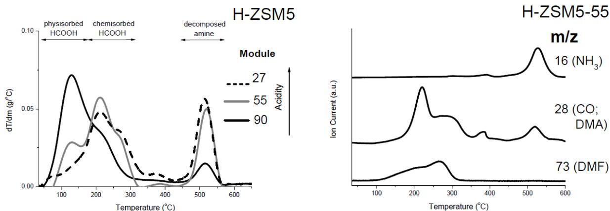
**Fig. 4** (LEFT) TGA measurement differential data of H-ZSM5 catalyst with different module values, impregnated with dimethylformamide - DMF. (RIGHT) MS spectra of H-ZSM5-55, impregnated with dimethylformamide recorded during TGA tests. DMA – dimethylamine.
