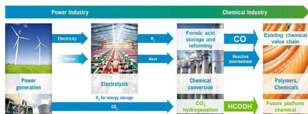
Formic acid could bridge the power and chemical industry sustainably integrating into the existing chemical value chain.
