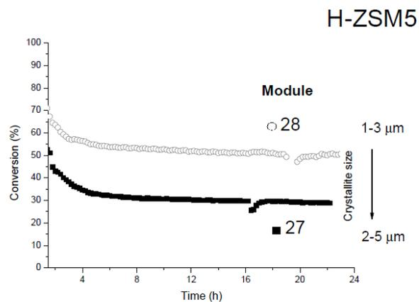
**Fig. 9** Diethylformamide conversion versus time on stream over H-ZSM5-27 and H-ZSM5-28 catalyst with different crystallite sizes. Test temperature 280°C, 0.6g catalyst, DEF flow 0.5mL/h.
