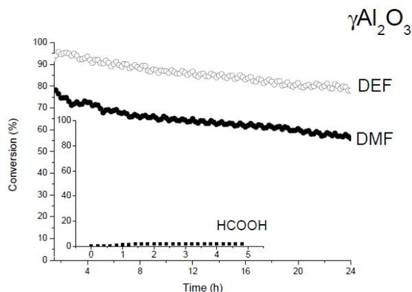
**Fig. 6** Conversion of different substrates (formic acid 98%-HCOOH; dimethylformamide-DMF; diethylformamide-DEF) versus time on stream over  $\gamma Al_2O_3$ . Test temperature: 190°C for HCOOH; 280°C for formamides, 0.6g catalyst, substrate flow 0.5 mL/h.
