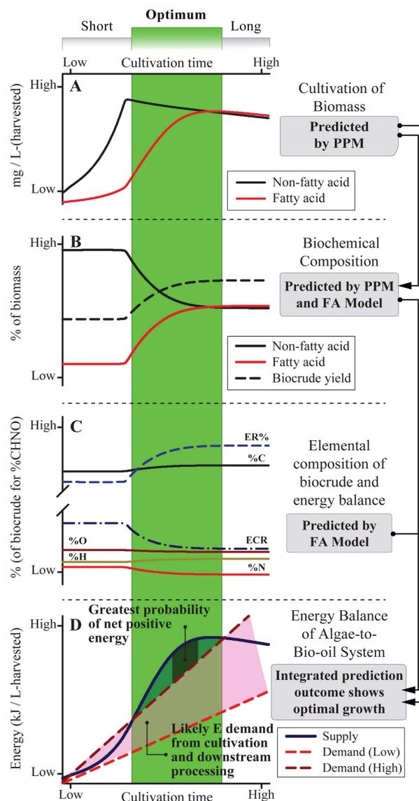
**Fig. 8** Results demonstrating the integrated modeling framework with cultivation time as the system variable. This demonstration is conceptual; quantitative analysis requires calibration of the PPM and FA models.
