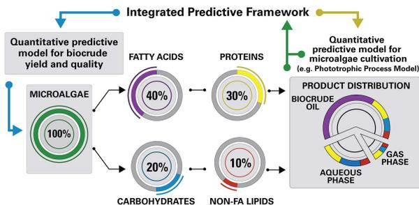
Models for microalgae hydrothermal liquefaction were developed from conversion of *Nannochloropsis* cultivated to varying biochemical composition and fatty acid content.
