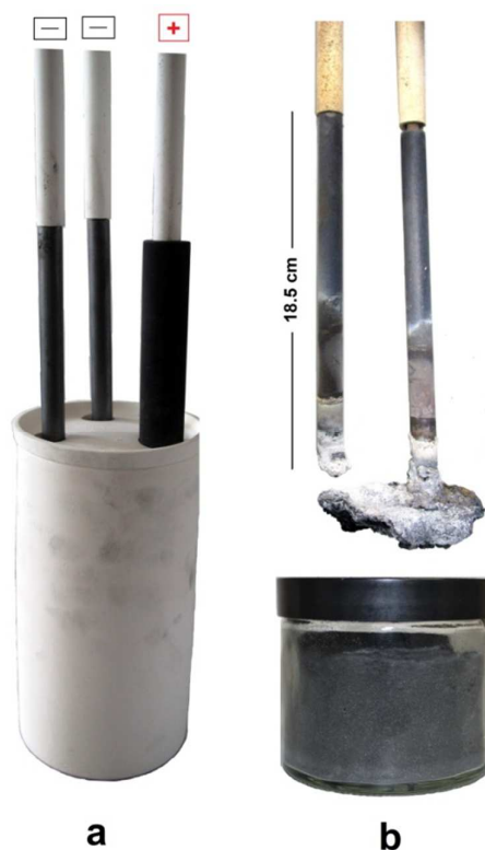
Fig. 5 (a) Photograph of the electrolysis cell. Two graphite rods served as alternative cathodes during the molten salt process. The arrangement of the electrodes in an alumina crucible containing LiCl, before loading into the molten salt reactor can be seen. (b) Photograph of the graphite electrodes after being used as cathode during the molten salt process. Part of the graphite cathodes exposed to the molten salt (about 11.5 cm) was completely exfoliated into graphene. Distilled water was added to the alumina crucible in order to dissolve the solidified LiCl, resulting in the retrieval of 70g graphene material, which was stored in a jar after vacuum filtration and drying.
