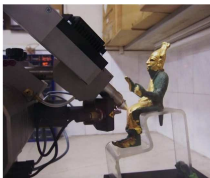
Figure 2: The head of the micro XRF spectrometer (ARTAX, Bruker Nano GmbH) during a measurement of the bronze figurine 1 at the Conservation laboratory of the National Archaeological museum of Damascus
