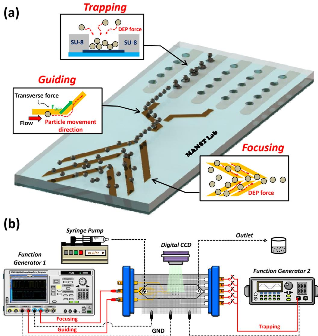
**Fig. 1** (a) Schematic diagram of three step DEP manipulations for focusing, guiding and trapping of nanoprobes for improved immunosensing efficiency. (b) Schematic of programmable control of DEP manipulations using function generators and detection of fluorescent response using digital CCD camera mounted on a microscope.
