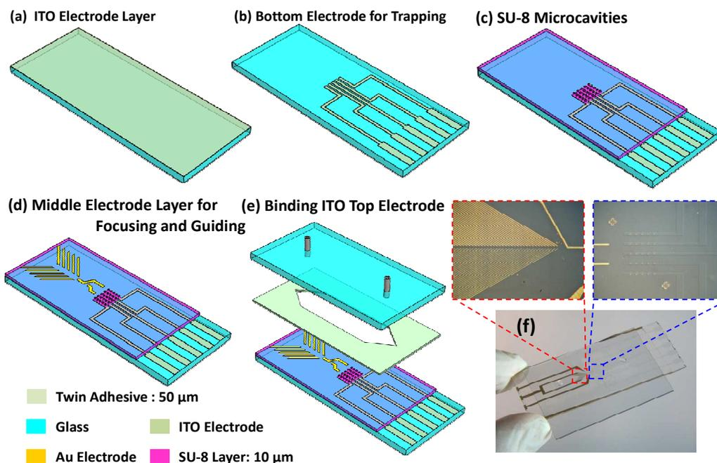
**Fig. 3** (a-e) Schematic of step by step fabrication for multiplexed immunosensing on a single LOC. (f) Image of completed device with enlarged images of patterned middle gold electrodes and bottom ITO electrodes as observed under an optical microscope.
