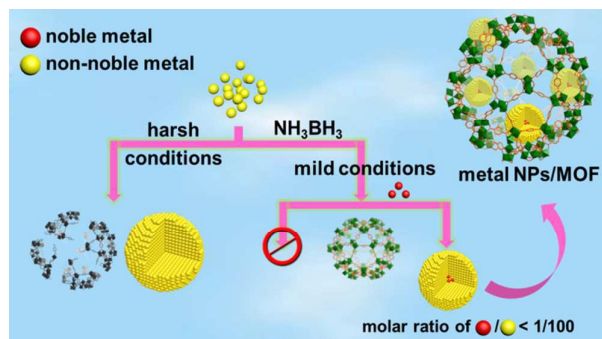
Scheme 1. Schematic illustration showing the preparation of non-noble metal NPs under harsh conditions or via a NMSM synthetic approach with moderate \text{NH}_3\text{BH}_3 under ambient conditions.
