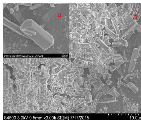
Fig. 5 SEM image of low magnification (A) and high magnification (a) of as-synthesized Cd-MOF-2
