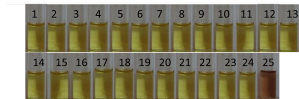
Fig. 3: (a) Absorbance spectra of Sdglu-Ag NPs in the absence of melamine (red line), with other analytes ( 5 \times 10^{-5} M) (black lines) and with melamine ( 5 \times 10^{-5} M) (blue line); (b) Photograph of colour change from yellow to red in melamine ( 5 \times 10^{-5} M) induced aggregated Sdglu-Ag NPs; (c) Photograph of colour change of Sdglu-Ag NPs with various other analytes ( 5 \times 10^{-5} M) (1. Sdglu-Ag NPs, 2. Gly, 3. Ala, 4. Leu, 5. Ile, 6. Phe, 7. Glu, 8. Arg, 9. His, 10. Trp, 11. Tyr, 12. Ser, 13. Lys, 14. Asp, 15. Met, 16. Cys, 17. Ascorbic acid, 18. Resorcinol, 19. Catechol, 20. Gallic acid, 21. Pyrogallol, 22. \text{Na}^+ , 23. \text{K}^+ , 24. \text{Ca}^{2+} , 25. Melamine)
