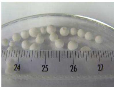
**Figure 2:** Obtained ferrocene functionalized ZnO nanoparticles formulated as beads
