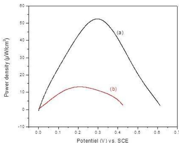
**Figure 9:** Power density plots of a glucose/air fuel cell using C/Pt as cathode catalyst and (a) ZnO-Fc/CNTs/GOx or (b) Fc/CNTs/GOx as anode catalyst. The flow rate of glucose is of  $5 \text{ mL min}^{-1}$  and the cathode operates under air conditions
