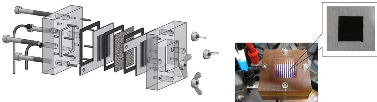
**Figure 8:** Schematic representation and image of the glucose/air fuel cell
