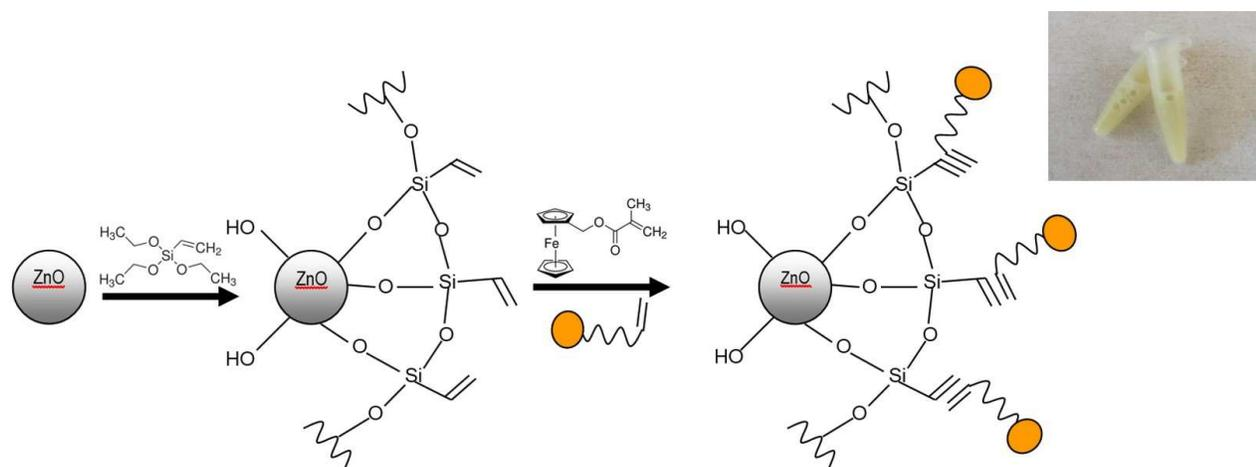
**Scheme 1:** Mechanism for the ZnO nanoparticles functionalization by the ferrocene redox mediator; (inset): image of the ZnO-Fc based dispersion in water
