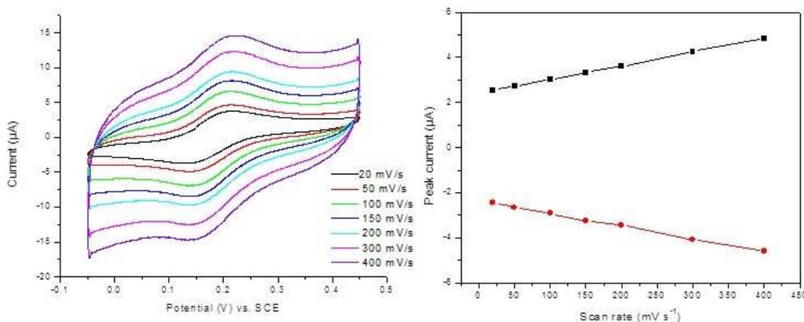
**Figure 6:** Left: Cyclic voltammogram of ZnO-Fc/CNT on glassy carbon electrode in 0.1 M phosphate buffer solution (pH 7) at 20, 5, 100, 150, 200, 300 and 400 mV s<sup>-1</sup> scan rate. Right: Anodic and cathodic peak current *versus* the scan rate for ZnO-Fc/CNT on glassy carbon electrode
