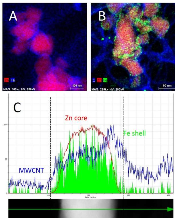
**Figure 4:** XEDS analysis of ferrocene-modified ZnO nanoparticles both (A) isolated and (B) supported on carbon nanotubes. (C) Linescan reveals the abundance of ferrocene on the surface
