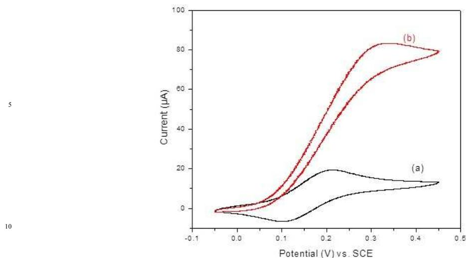
**Figure 7:** Cyclic voltammogram of ZnO-Fc/CNT/GOx on glassy carbon electrode in 0.1 M phosphate buffer solution (pH 7) (a) in absence and (b) in presence of glucose. Scan rate:  $50 \text{ mV s}^{-1}$ .
