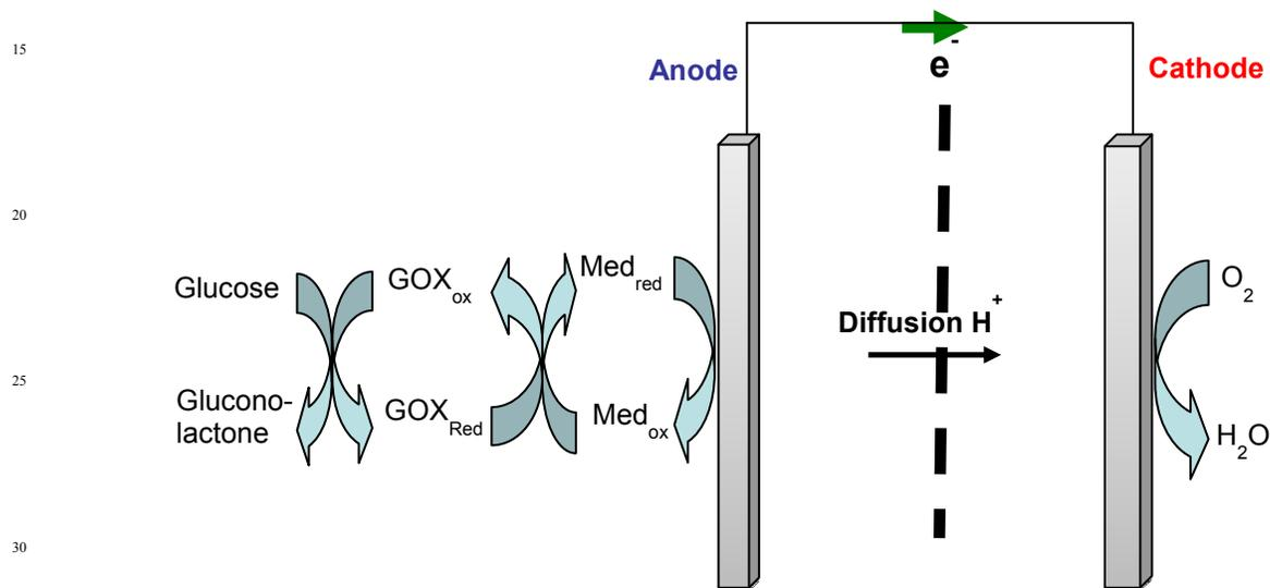
Figure 1: Principle of the bio-fuel cell described in the present manuscript
