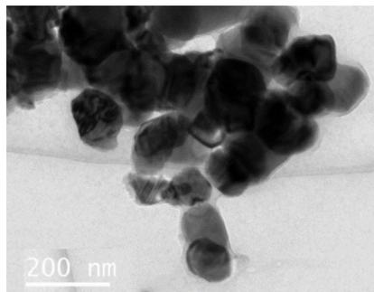
**Figure 3:** TEM micrograph of the ZnO-Fc nanoparticles
