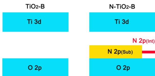
Figure 6. Scheme of the band structures of the pure and N-doped TiO 2 -B.
