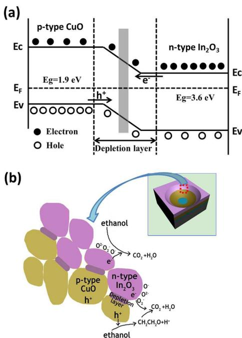
**Fig. 5** the schematic energy band diagram of the p-CuO/n- $\text{In}_2\text{O}_3$  hetero-junction at thermal equilibrium and the sensing mechanism schematic model for the p-CuO/n- $\text{In}_2\text{O}_3$  based sensor when it exposes to ethanol gas
