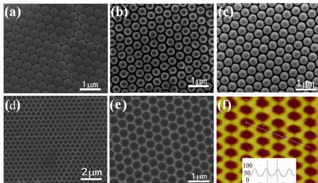
**Fig. 2** SEM images of self-assemble PS template (a), PS template after plasma etching (b), etched PS template after magnetron sputter deposition (c) and after ultrasonic washing (d) (e), AFM image of  $\text{In}_2\text{O}_3/\text{CuO}$  bilayer porous thin film (f).
