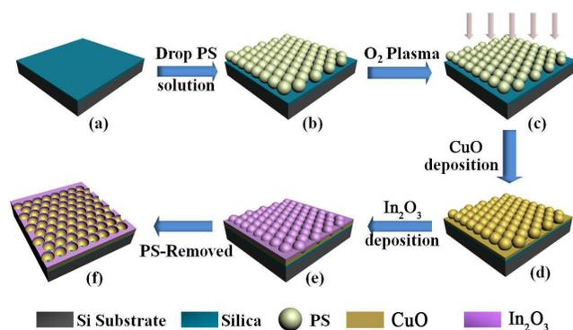
**Fig. 1** the schematic of the side view of uniform  $\text{In}_2\text{O}_3/\text{CuO}$  bilayer porous thin film.
