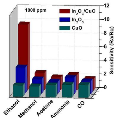
**Fig. 4** Sensitivity of  $\text{In}_2\text{O}_3$ ,  $\text{CuO}$  single layer porous film and  $\text{In}_2\text{O}_3/\text{CuO}$  bilayer porous thin film to 1000 ppm different gases at 250 °C.
