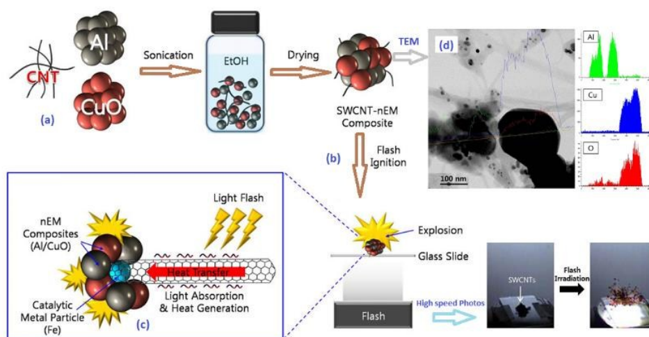
Figure 37, Schematics of (a) the fabrication of SWCNT-nEM composites, (b) the flash ignition of an SWCNT-nEM composite, (c) the optical ignition mechanism of an SWCNT-nEM composite, and (d) scanning TEM image and line scan analysis of SWCNT/Al/CuO nanocomposites. Recombination of several figures from Ref. 280 with permission of Copyright © 2012 The Combustion Institute. Published by Elsevier Inc.
