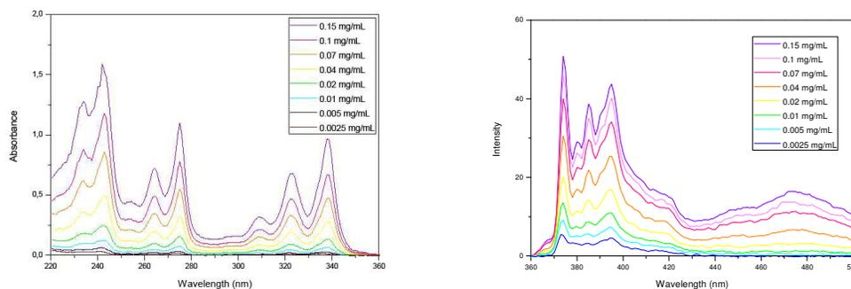
**Figure 7.** (a) UV-Vis spectra of pyrene in C12-HBPE-ABS (left) and (b) Fluorescence spectra of pyrene in C12-HBPE-ABS (right).
