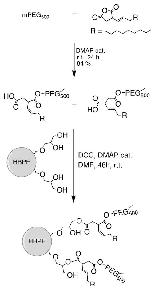
**Scheme 2.** Synthesis of the core-ABS nanocarrier: Schematic synthesis of the amphiphilic shell and further reaction with the hyperbranched polyesters.
