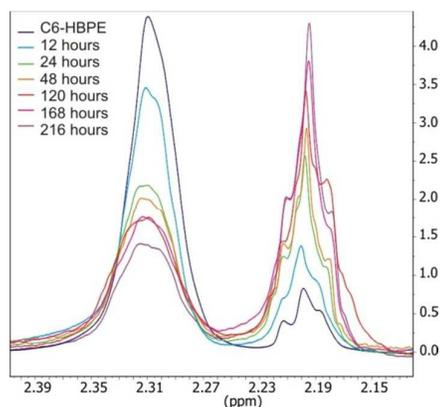
**Figure 2.** <sup>1</sup>H-NMR magnification of the protons in alpha position to the carbonyl groups of C6-HBPE during the degradation process in presence of CALB at 37°C. Signal at 2.32 ppm is related to the ester and 2.20 ppm is related to the carboxylic acid.
