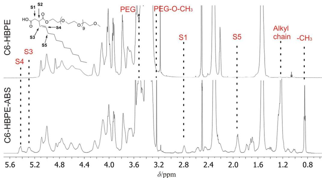
**Figure 4:** <sup>1</sup>H-NMR spectra comparison between C6-HBPE and C6-HBPE-ABS.
