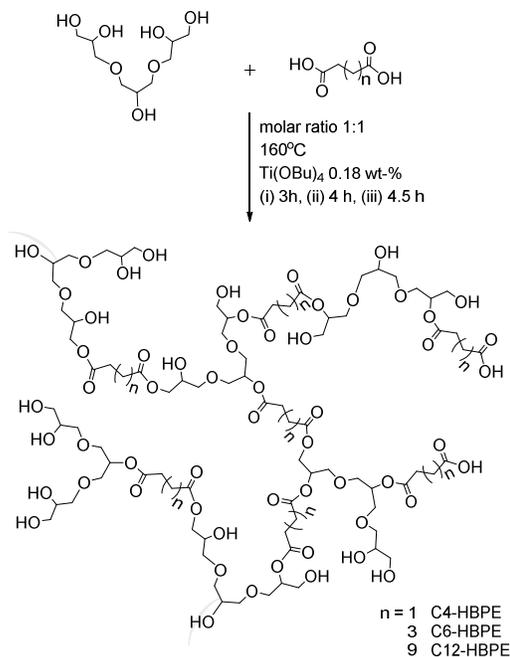
**Scheme 1.** Synthesis of the HBPEs and schematic representation of the HBPEs. (i) C4-HBPE, (ii) C6-HBPE, (iii) C12-HBPE.
