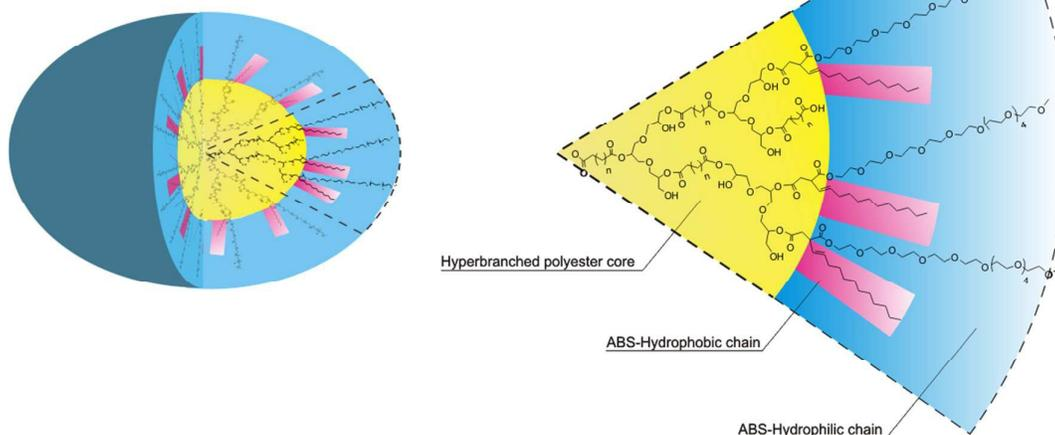
**Figure 3:** Schematic representation of the Core-ABS nanocarrier
