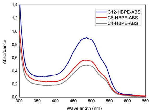
**Figure 11.** UV-Vis spectra of DOX loaded in 1 mg/mL solution in PBS of C4-HBPE-ABS, C6-HBPE-ABS and C12-HBPE-ABS.
