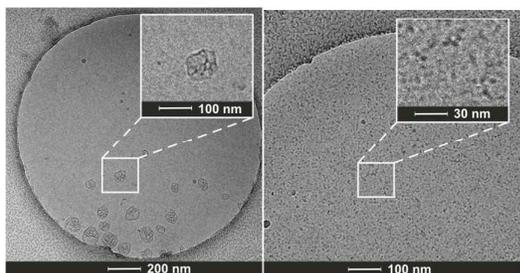
**Figure 5.** Cryo-TEM microscopic images of C12-HBPE-ABS in water (left) and C6-HBPE-ABS in water (right).
