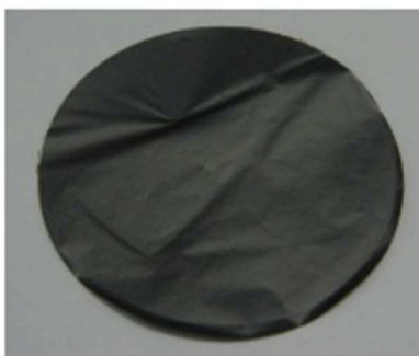
Fig. 1 Digital photograph of free-standing r-GO paper. 55x47mm (96 x 96 DPI)
