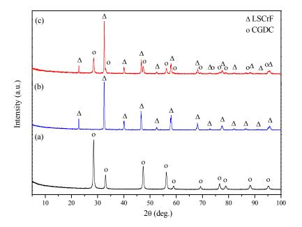
Fig. 2 XRD patterns of (a) pure CGDC; (b) pure LSCrF; (c) LSCrF-CGDC composite cathode fired at 700 °C
