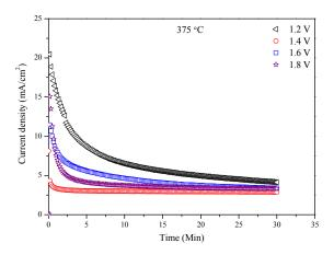
Fig. 8 Electrolytic cell performance stability at 375 °C and 1.2-1.8 V
