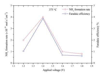
Fig. 9 Dependence of the rate of ammonia formation rate on the applied voltage at 375 °C
