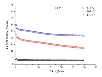
Fig. 5 Electrolytic cell performance stability at 1.4 V and 375-425  $^{\circ}$ C.
