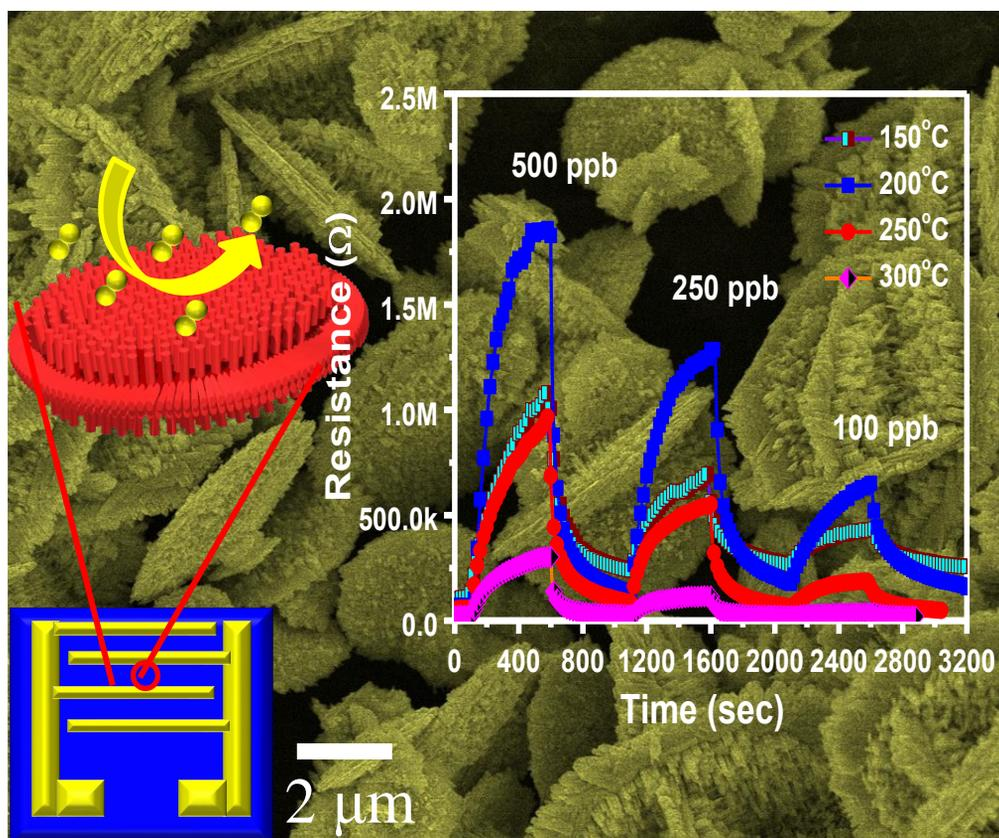
Gas nanosensor based on Micro-wheels composed of self-assembled tungsten oxide nanorods exhibited excellent sensing performance to ppb level Cl<sub>2</sub>
