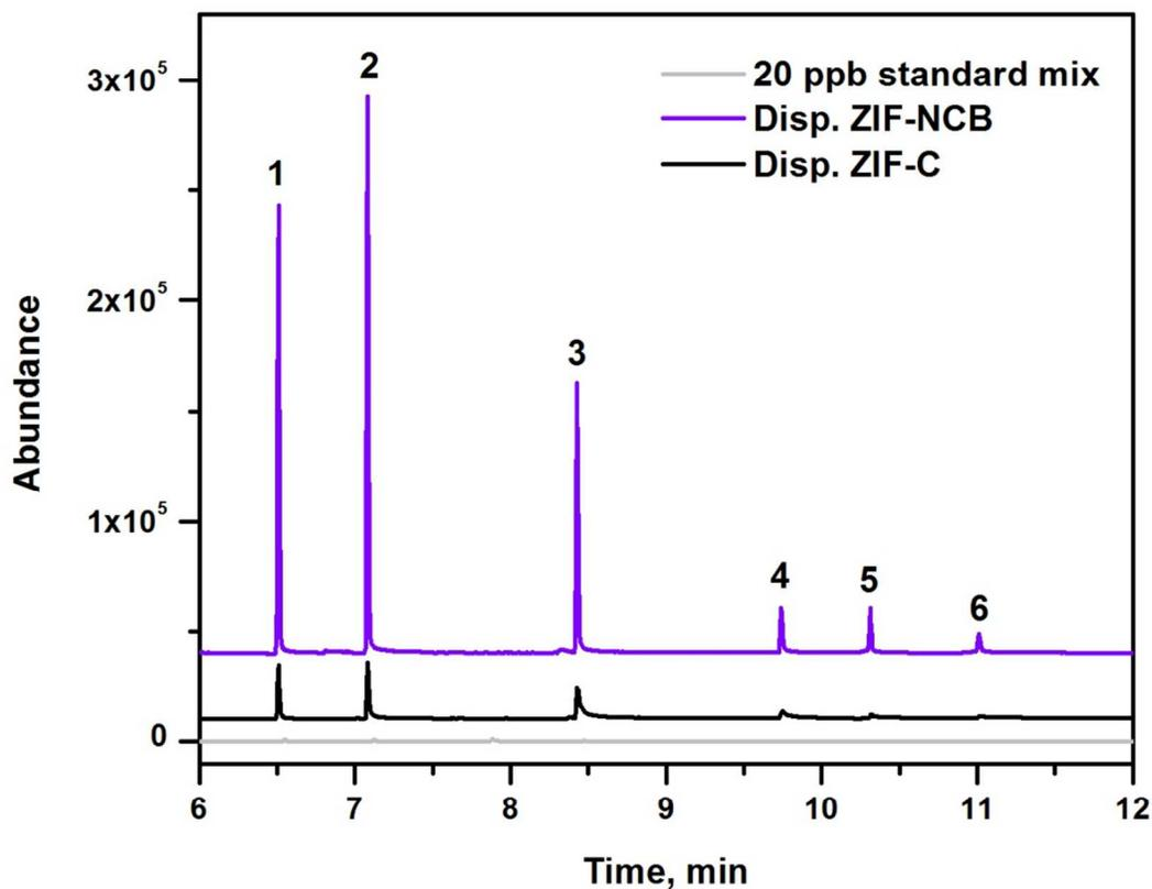
**Fig. 6** GC-MS chromatograms of a mixture of 6 phthalate esters obtained by direct injection of a 20  $\mu\text{g/L}$  standard and after solvent-assisted porous solid sorbent extraction using the larger ZIF-8 microcrystals (ZIF-C) and the ZIF-8 nanocrystals synthesized using *n*-butylamine as modulator agent (ZIF-NCB). Peaks: 1, DMP; 2, DEP; 3, DBP; 4, DEHP; 5, BBP; 6, DNOP.
