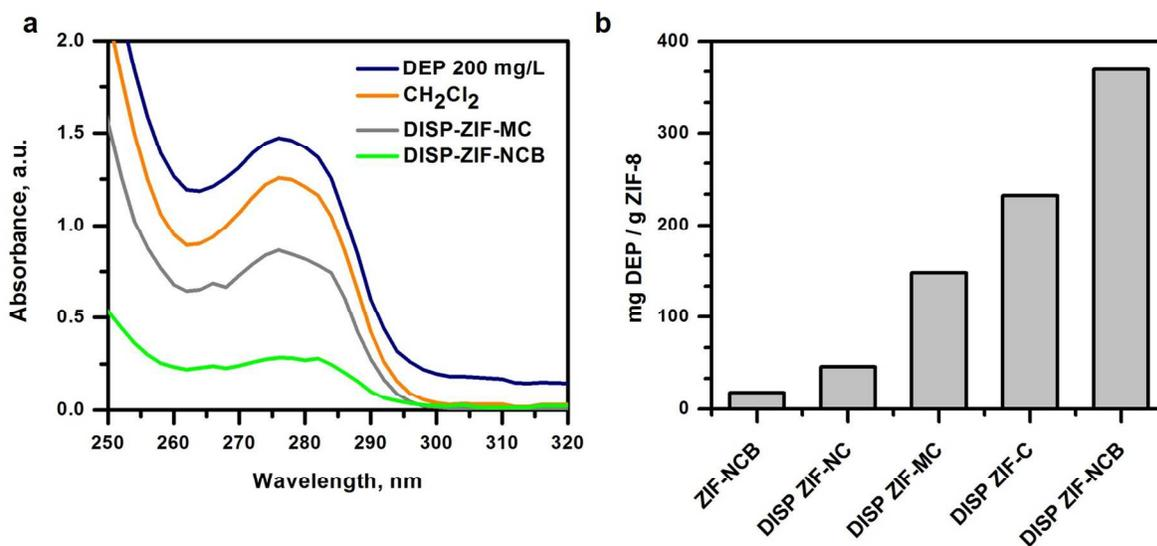
**Fig. 4** a) UV-vis spectra of a 200 mg/L diethyl phthalate (DEP) solution before and after extraction with a dispersion without ( $\text{CH}_2\text{Cl}_2$ ) and with 5 mg/mL of both ZIF-8 microcrystals (DISP-ZIF-MC) and ZIF-8 nanocrystals synthesized using *n*-butylamine as modulator agent (DISP-ZIF-NCB). b) Quantification of the amount of DEP extracted by using different ZIF-8 crystals. The contribution of DEP extraction by the dichloromethane/methanol mixture has been
