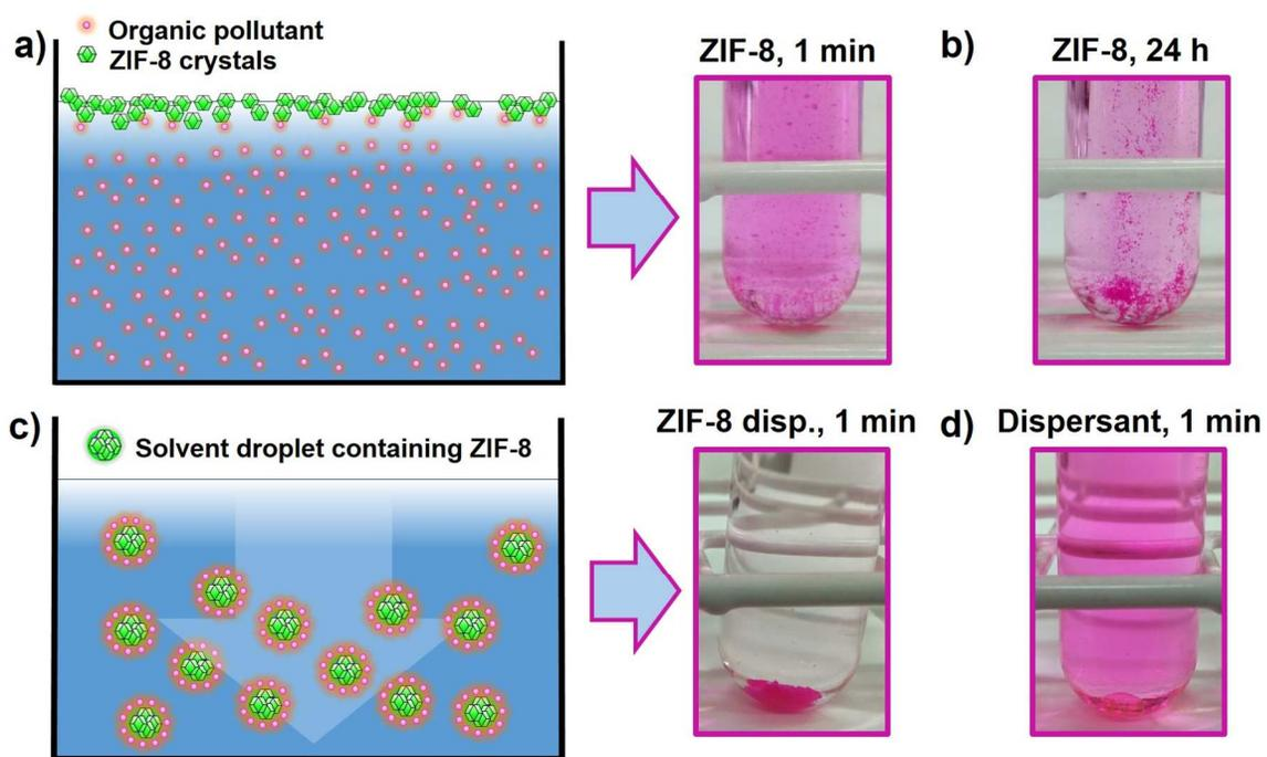
**Fig. 1** Extraction of rhodamine B ( $10 \mu\text{M}$ ,  $9 \text{ mL}$ ) in water by direct addition of ZIF-8 crystals after a) 1 h and b) 24 h. Addition of c) an identical amount of ZIF-8 crystals dispersed in 1 mL of a dichloromethane/methanol mixture (20/80, v/v%), and d) an identical solvent mixture in the absence of ZIF-8 crystals.
