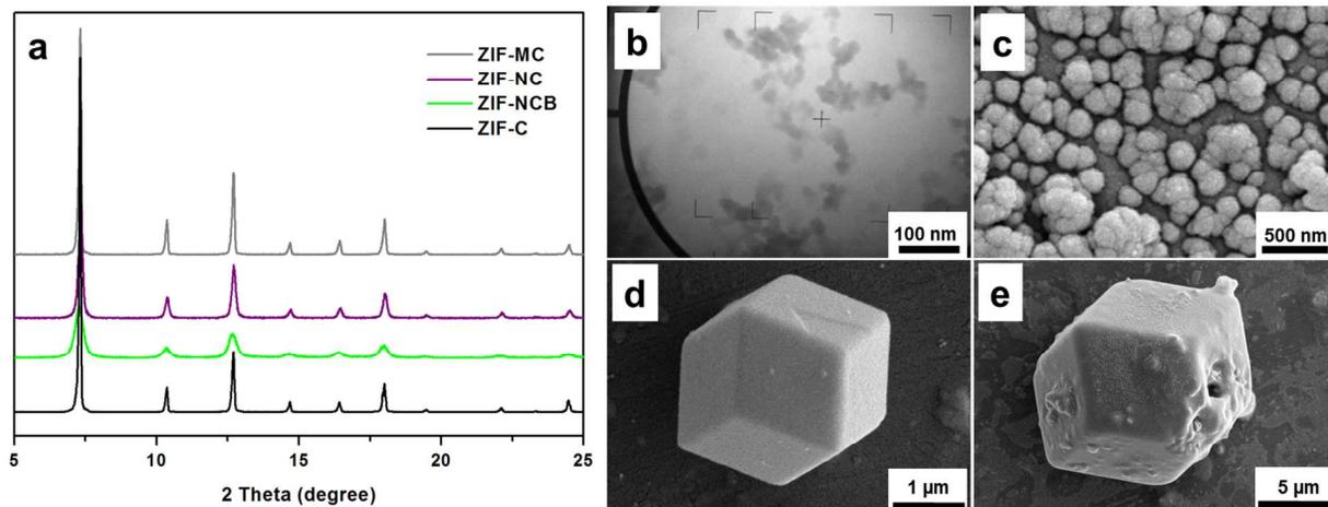
**Fig. 2** a) Powder X-ray diffraction patterns of the different ZIF-8 samples synthesized: ZIF-NCB, *n*-butylamine modulated nanocrystals; ZIF-NC, nanocrystals; ZIF-MC, formate modulated microcrystals; and ZIF-C, formate modulated microcrystals prepared at 373 K. TEM image of ZIF-NCB (b). SEM images of ZIF-NC (c), ZIF-MC (d), and ZIF-C (e).
