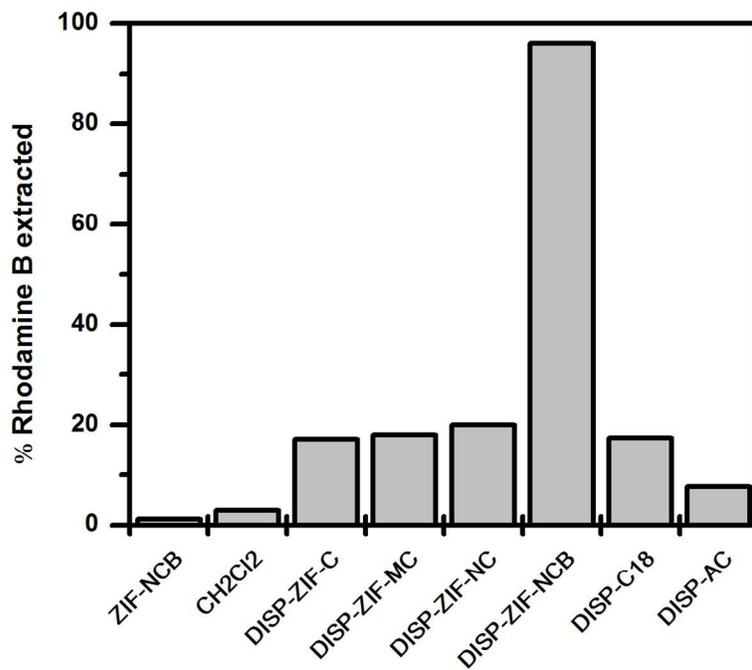
**Fig. 3** Percentage of Rhodamine B extracted using dispersions of ZIF-8 crystals of different size. Results obtained using only the solvent mixture (CH<sub>2</sub>Cl<sub>2</sub>), only the butylamine-modulated ZIF-8 crystals (ZIF-NCB) and dispersions of activated carbon (DISP-AC) and silica-C18 beads (DISP-C18) are also shown for the sake of comparison. See experimental section for details on the extraction procedure.
