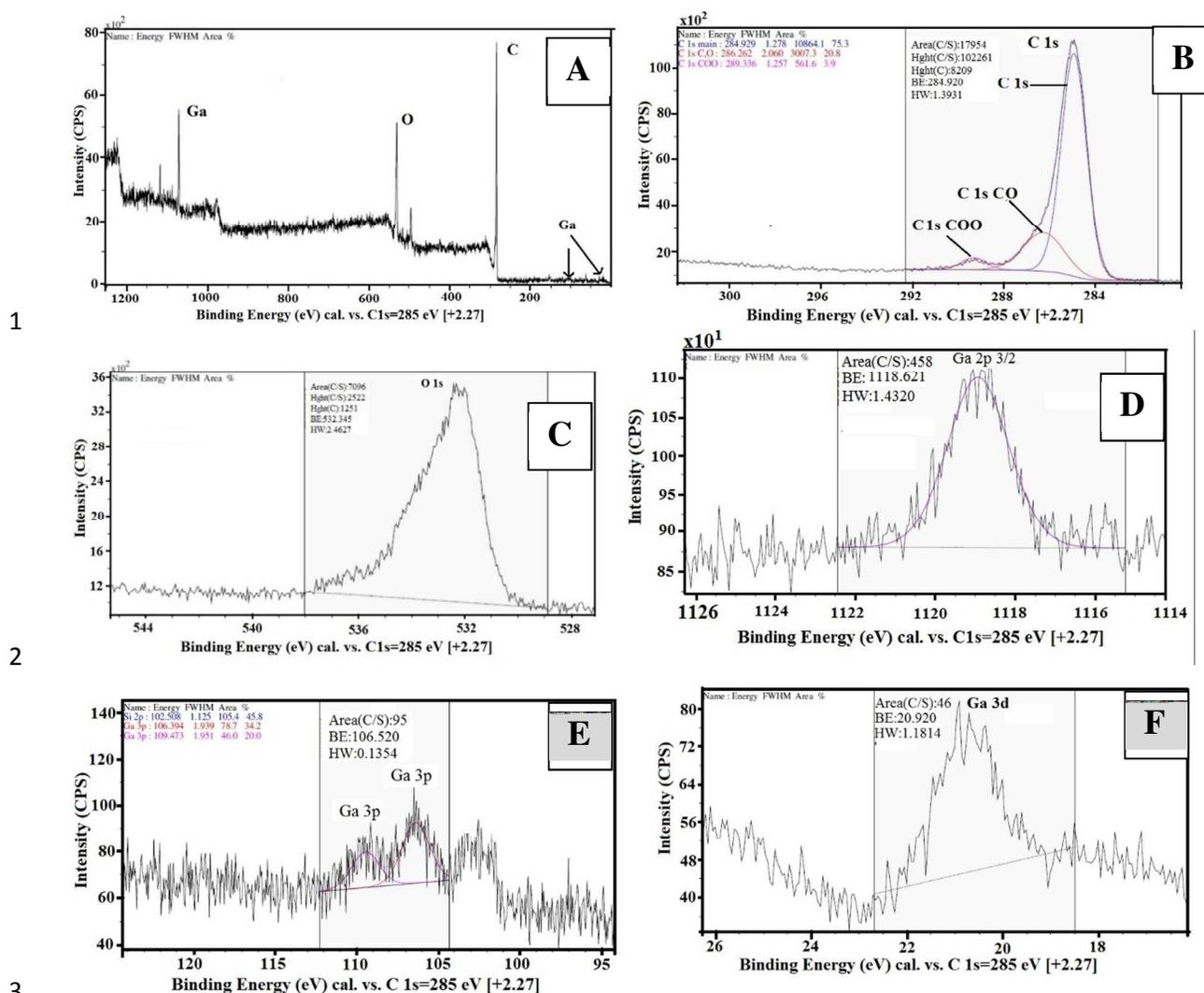
**Fig. 6.** (A) Full XPS spectrum, (B) XPS spectrum of C 1s, (C) XPS spectrum of O 1s, (D) XPS spectrum of Ga 2p (E) XPS spectrum of Ga 3p and (F) XPS spectrum of Ga 3d of Ga@C-dots.
