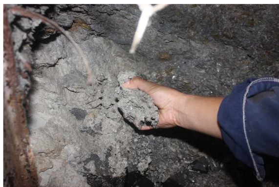
Fig. 12 Macroscopic argillization and liquefaction in the mudstone at the Lihai mine.
