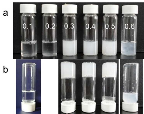
Fig. 1 Macroscopic appearance (a) and the tube inversion test (b) of HDPS/SDS mixed surfactant solutions ( C_T=100 \text{ mmol}\cdot\text{L}^{-1} ). The numbers in the photos are the molar percentages of SDS ( X_{\text{SDS}} ).
