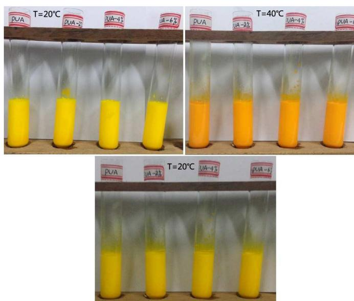
Fig. 11. Thermochromic effect of the waterborne UV-curable thermochromic coatings with different SiO<sub>2</sub> content.
