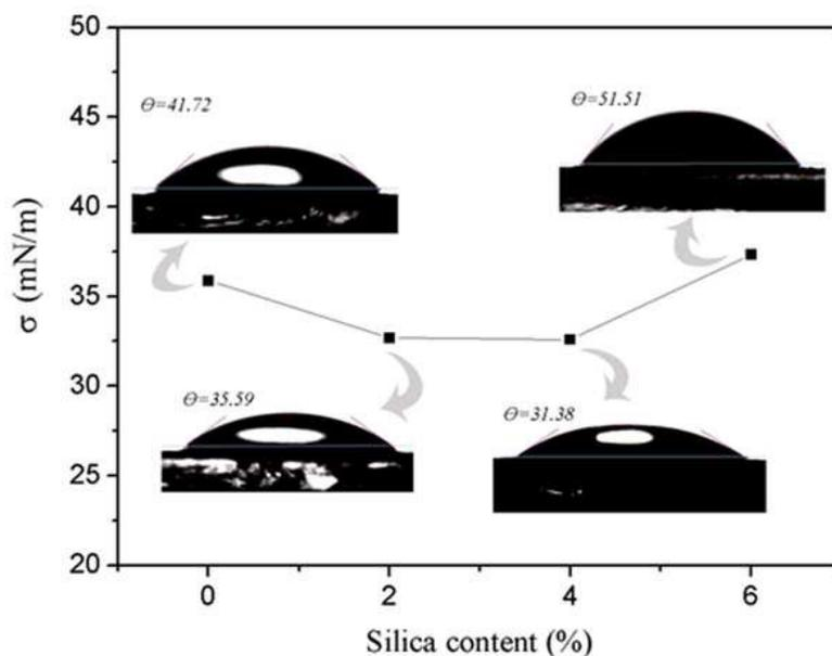
Fig. 5. Surface tension ( $\sigma$ ) curve and contact angle ( $\theta$ ) images of PUA/ $\text{SiO}_2$  nanocomposites with different  $\text{SiO}_2$  content.
