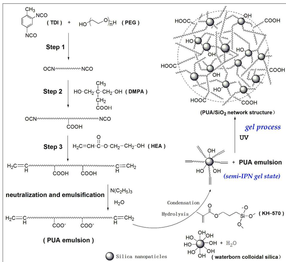
Fig. 1 Synthesis scheme to prepare PUA and PUA/SiO<sub>2</sub> nanocomposite.
