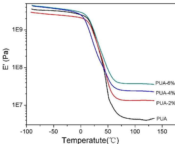
Fig. 7. Storage modulus  $E'$  in dependence on temperature for the PUA/SiO<sub>2</sub> nanocomposites films.
