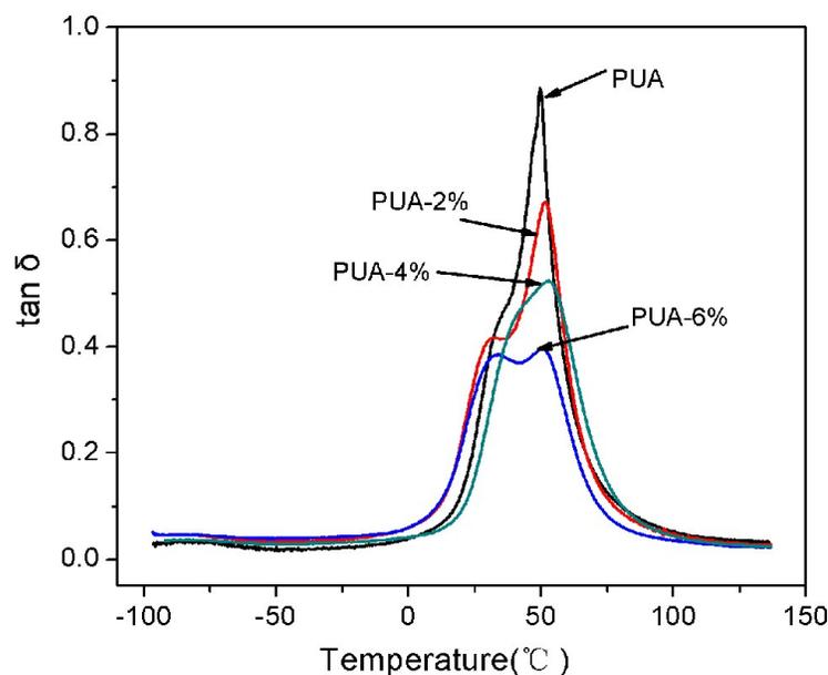
Fig. 8. Isochronal temperature dependence of  $\tan\delta$  for the PUA/SiO<sub>2</sub> nanocomposites films.
