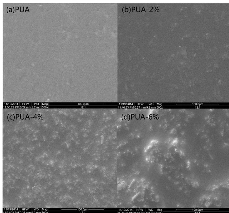
Fig. 4. SEM diagrams of the hybrid films: (a) pure PUA, (b) PUA with 2 wt% modified SiO<sub>2</sub>, (c) PUA with 4 wt% modified SiO<sub>2</sub> and (d) PUA with 6 wt% modified SiO<sub>2</sub>.
