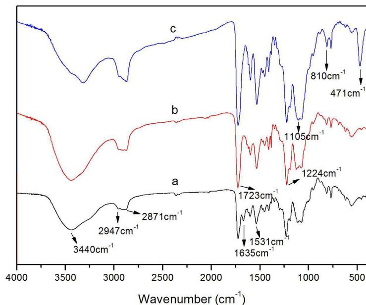
Fig. 2. FTIR spectra of PUA and hybrid film: (a) PUA emulsion, (b) PUA cured film, (c) PUA/ $\text{SiO}_2$  cured film with 4 wt%  $\text{SiO}_2$ .
