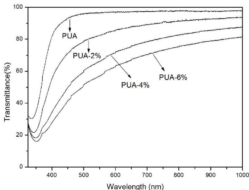
Fig. 9. UV-vis spectra of PUA and PUA/SiO<sub>2</sub> films with the thickness of 300 μm.
