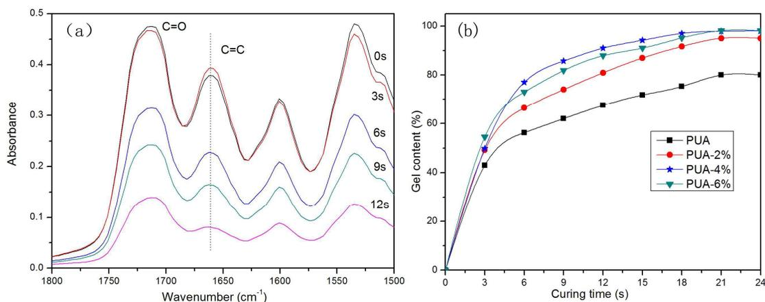
Fig. 6. The ATR-FTIR (a) of PUA film and gel content (b) of hybrid coatings at different curing time.
