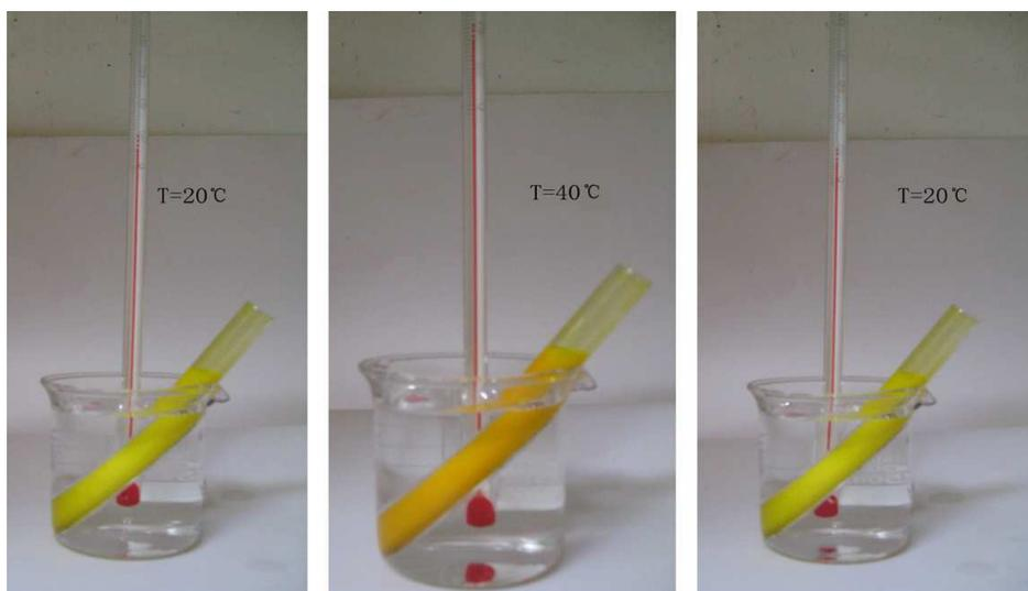
Fig. 10. Thermochromic effect of the waterborne UV-curable thermochromic coating.
