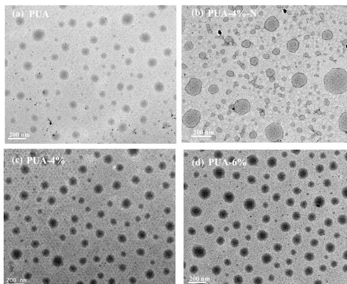
Fig. 3. TEM micrographs of PUA and PUA/SiO<sub>2</sub> hybrids particles: (a) pure PUA, (b) PUA with 4 wt% unmodified SiO<sub>2</sub>, (c) PUA with 4 wt% modified SiO<sub>2</sub> and (d) PUA with 6 wt% modified SiO<sub>2</sub>.
