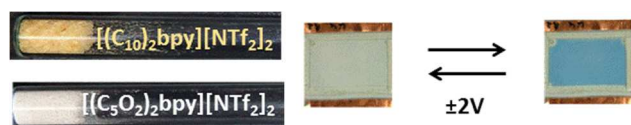
Figure 4 – Switch of colours of the different symmetrical disubstituted bipyridinium salts combined with Bis(trifluorometanesulfonyl)imide.
