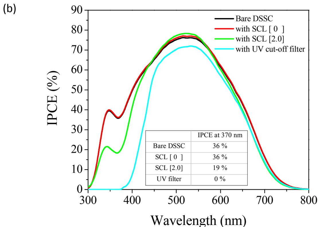
Fig. 3 (a) Initial Photo-to-Current conversion efficiencies and (b) Incident Photon-to-Current efficiencies (IPCE) of the prepared DSSCs using (i) bare FTO glass without any optical filter, (ii) 1,8-naphthaimide derivatives 0 and 2 wt.% as SCL and (iii) commercial UV cut-off filter, respectively.
