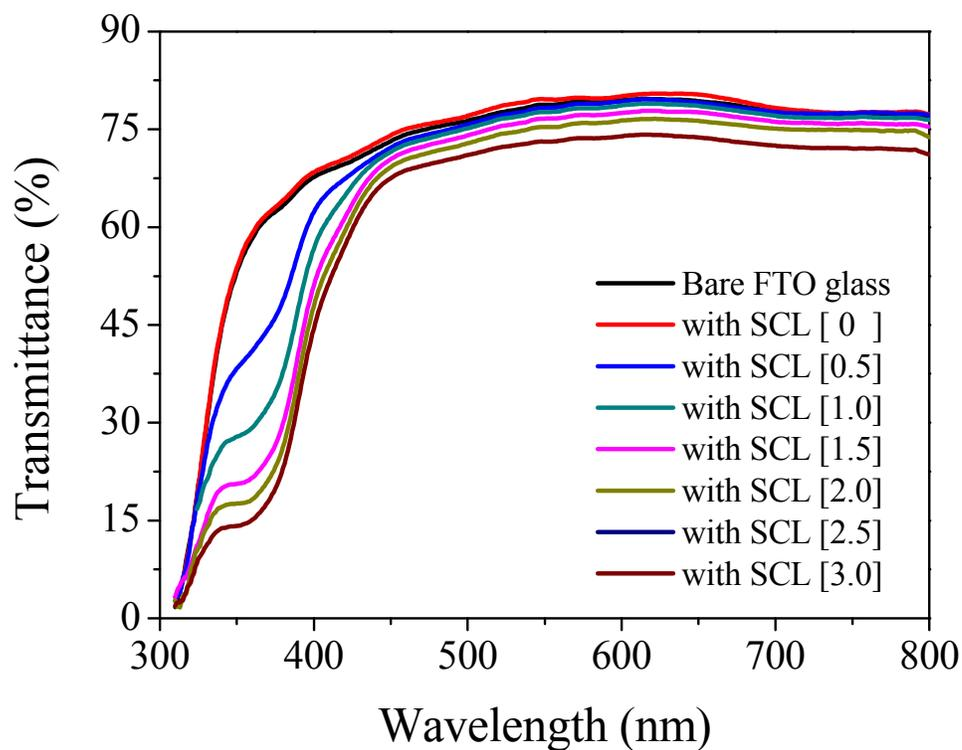
Fig. 1 Transmittances of FTO glasses with SCL of 0, 0.5, 1.0, 1.5, 2.0, 2.5 and 3.0 wt.% 1,8-naphthalimide derivatives, respectively.
