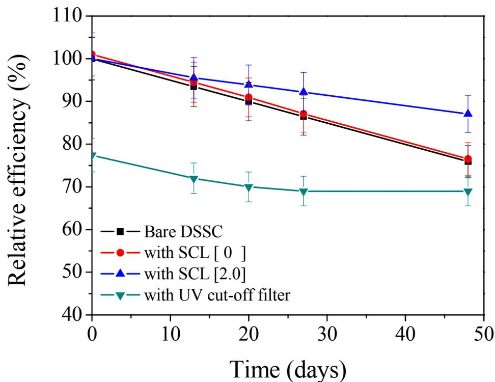
Fig. 4 Relative outdoor Photo-to-Current conversion efficiencies of the prepared DSSCs using (i) bare FTO glass without any optical filter, (ii) 1,8-naphthaimide derivatives 0 and 2 wt.% as SCL and (iii) commercial UV cut-off filter, respectively.
