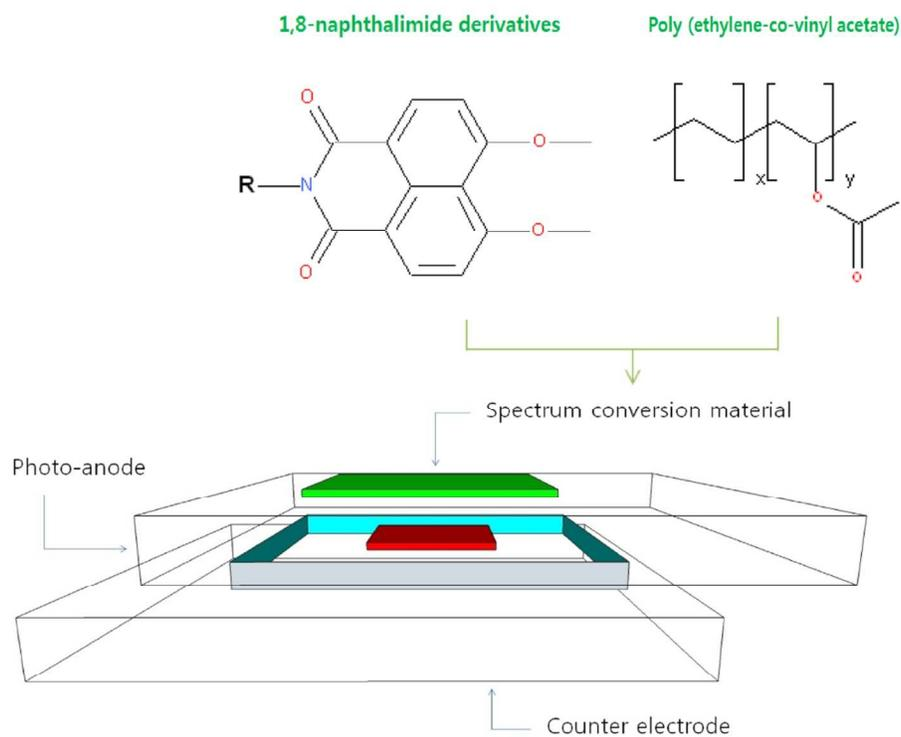
Scheme 1 Exciton complex forming spectrum conversion material with a compound of 1,8-naphthalimide derivatives in EVA (poly (ethylene-co-vinyl acetate)) is coated on the photo-anode of the DSSC.
