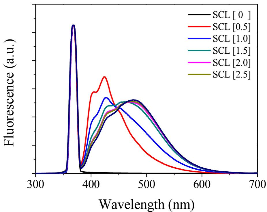
Fig. 2 Fluorescences of FTO glasses with SCL of 0, 0.5, 1.0, 1.5, 2.0, 2.5 and 3.0 wt.% 1,8-naphthalimide derivatives, respectively.
