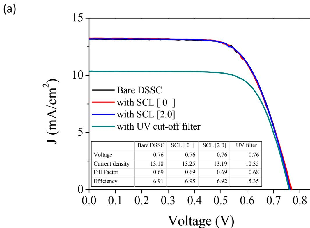
Fig. 3 (a) Initial Photo-to-Current conversion efficiencies and (b) Incident Photon-to-Current efficiencies (IPCE) of the prepared DSSCs using (i) bare FTO glass without any optical filter, (ii) 1,8-naphthaimide derivatives 0 and 2 wt.% as SCL and (iii) commercial UV cut-off filter, respectively.
