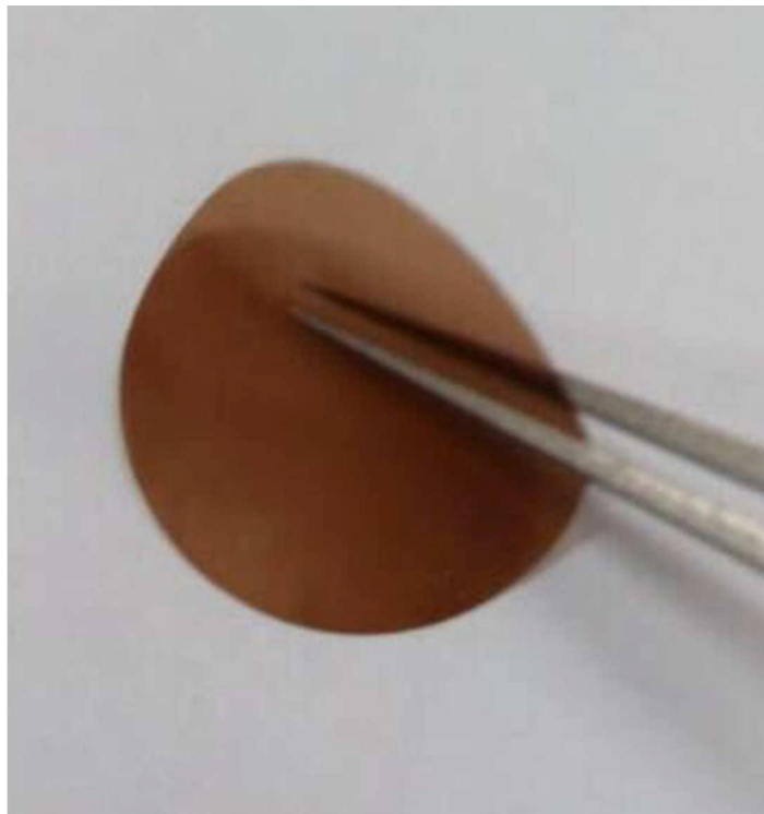
Fig. 1. The photograph of electrolyte membrane. 29x31mm (300 x 300 DPI)
