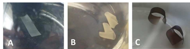
Fig. 6. Photographs of the samples L_{100K} (A) and D1_50 (B) after 48 hours of immersion at room temperature in the Pd(II) acetate solution, and D1_50 (C) immersed for 1 hour at 80 °C (all the samples were washed before the pictures).
