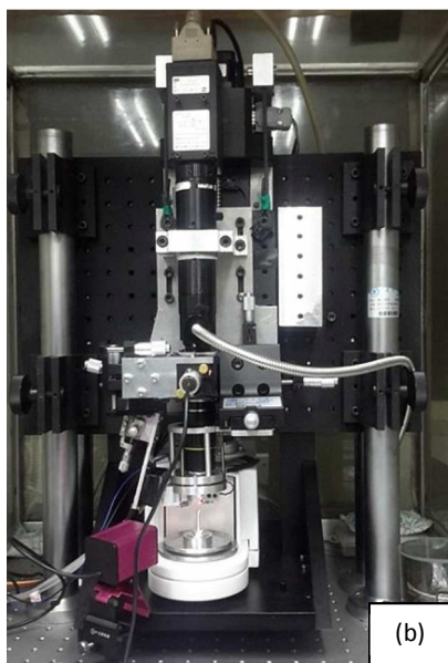
Fig. 1 (a) Schematically illustration of the spring constant calibration system. 1. Electromagnetic balance; 2. Sapphire plate; 3. Balance bracket; 4. Reflector; 5. Lens; 6. PSD; 7, 10. Ultra-precision 3D motor stages; 8. Laser diode; 9. Z-scanner; 11. Objective; 12, 13. Beam splitters; 14. Illuminator; 15. CCD; 16. Tube lens; 17. Z-axis motor stage; 18. Enclosure; 19. Vibration isolator; 20. Supporting breadboard; 21. Supporting columns. (b) Photo of the calibration system.
